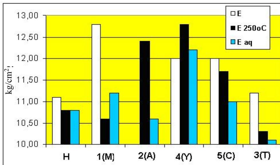
Figure 6: A comparative histogram of the values of the modulus of elasticity of compression of the samples at different exposure modes - the usual 60 °C; hard 250 °C and exposure in water for 7 days (Eq).
