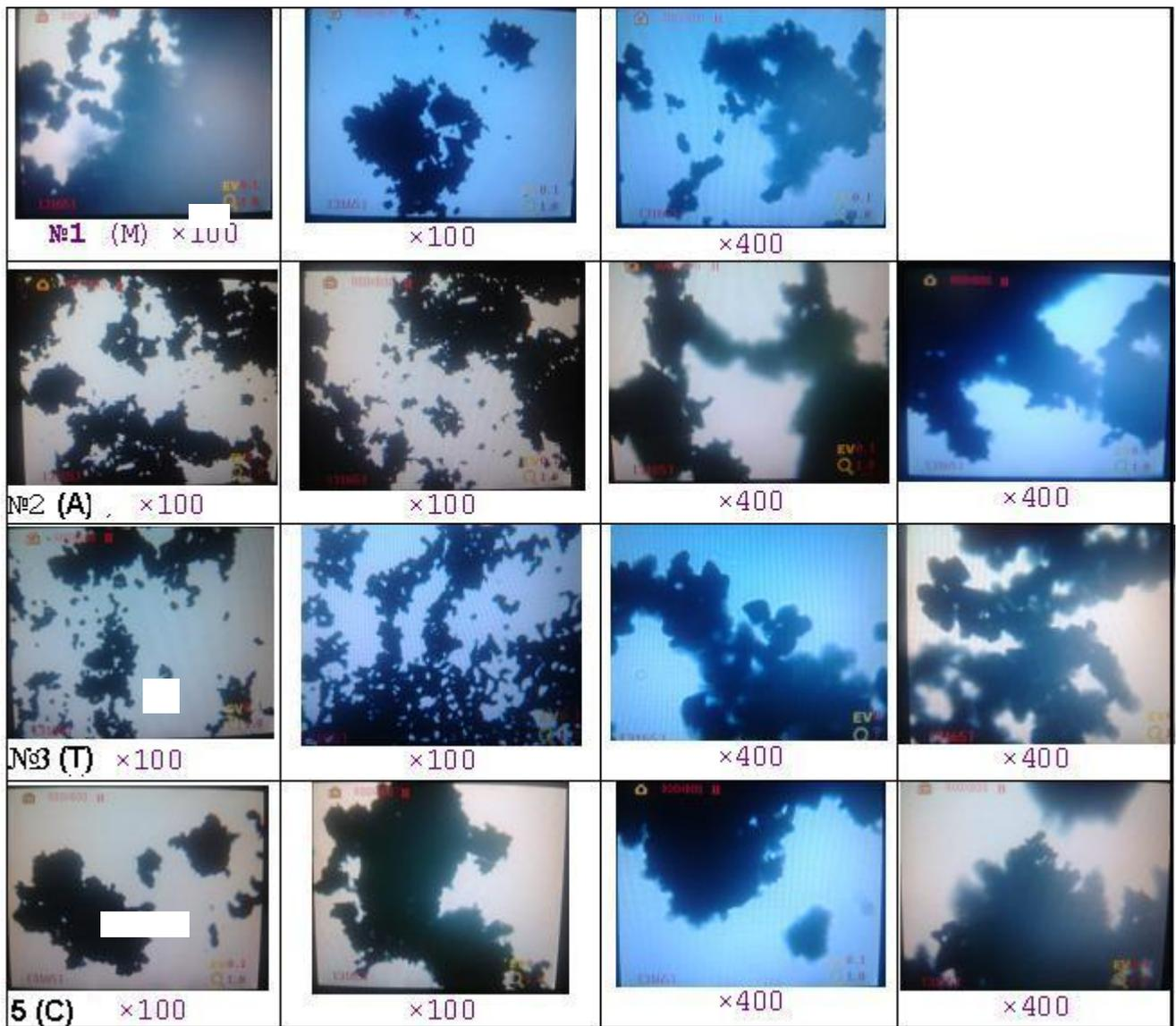
**Figure 2:** Optical microphoto of magnetite powders, with an increase of 100 or 400 times (with a screen length of 7 cm).
