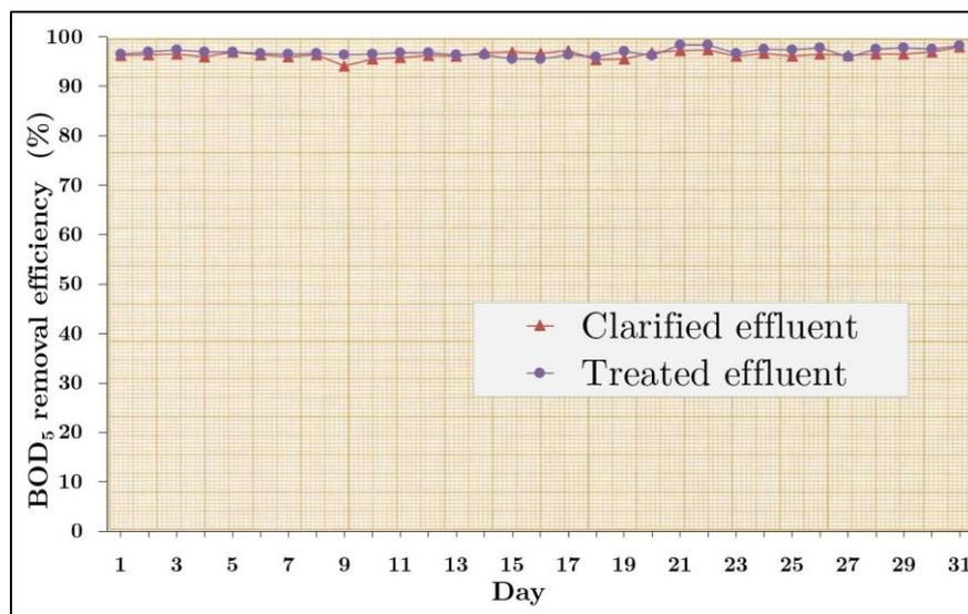
Figure 14: Steady-state BOD<sub>5</sub> removal efficiency in WWTP.
