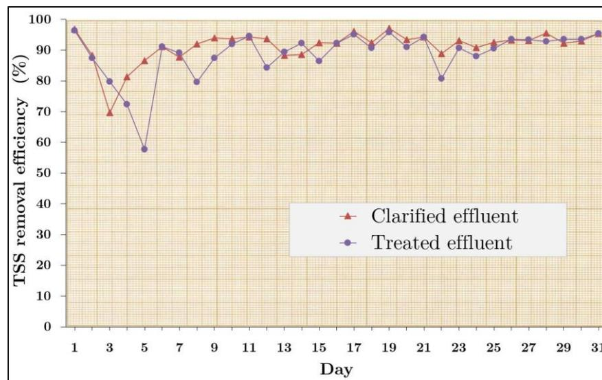
Figure 12: Steady-state TSS removal efficiency in WWTP.
