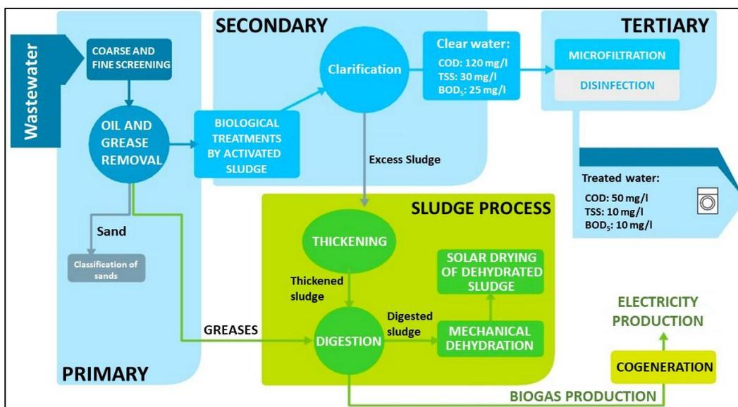
Figure 3: Diagram of the WWTP in Khouribga City.
