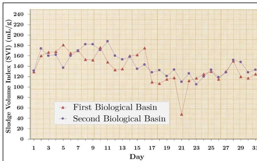
Figure 16: Sludge Volume Index changes in two biological basins of WWTP.
