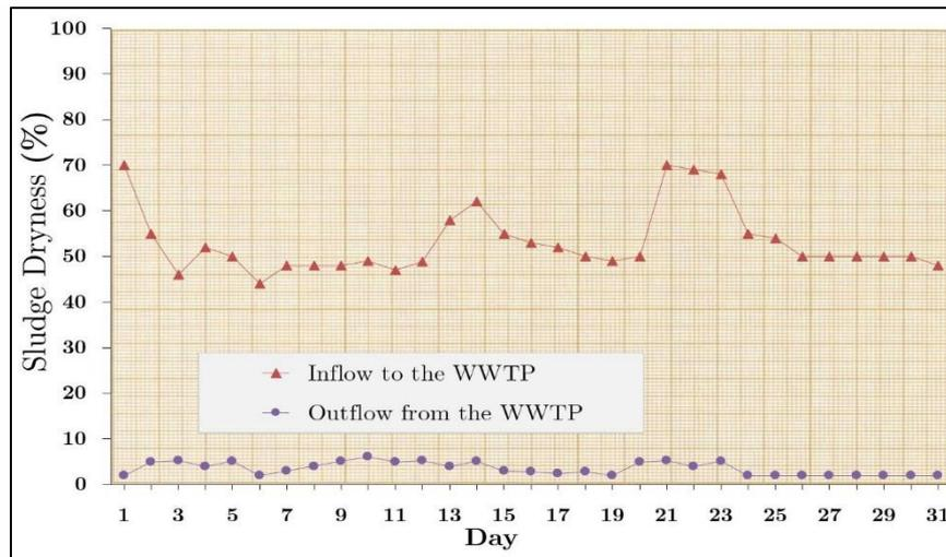
**Figure 17:** Rate change of sludge dryness in WWTP.
