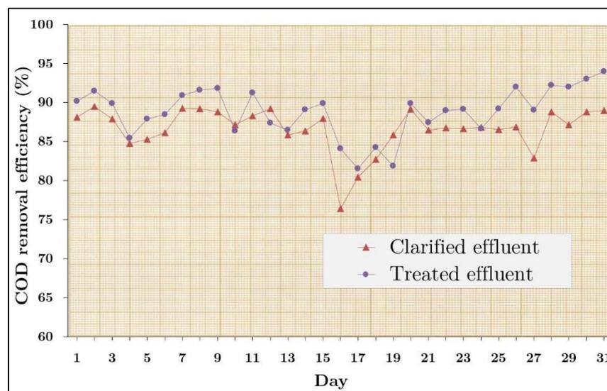
Figure 13: Steady-state CDO removal efficiency in WWTP.
