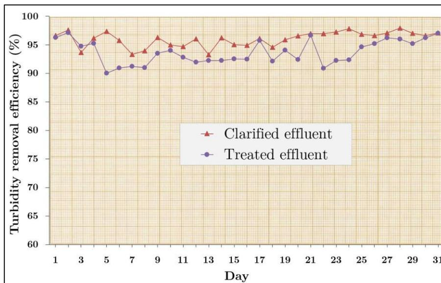
Figure 11: Steady-state Turbidity removal efficiency in WWTP.
