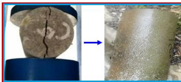
**Figure 7:** Test specimens during and after tensile test
