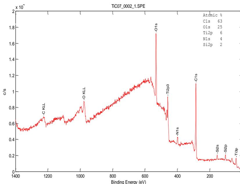
**Figure 12:** XPS survey on the unetched surface of a 488 nm TiC film deposited on silicon at 200 W. The atomic percentage of the elements at the surface are 63% C 1s, 25% O 1s, 6% Ti 2p, 4% N 1s and 2% for Si 2p.
