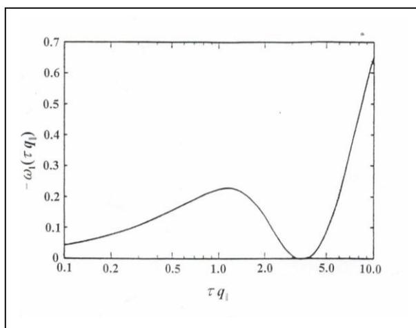
**Figure 1:** Rayleigh frequency shift due to surface roughness as a function of  $\tau q_{\parallel}$  (After Eguiluz and Maradudin [18]).
