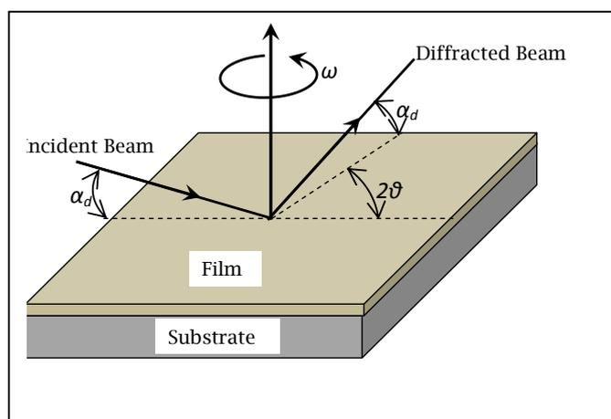
**Figure 9:** Schematic diagram of the GIXRD geometry.
