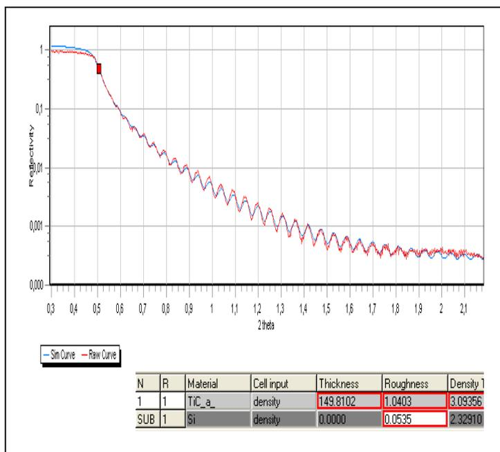
**Figure 7:** XRR measurement for a TiC film on silicon prepared at 100 W for 28 min. The fit parameters for the simulation curve are highlighted in red. The parameter values are: layer thickness 149.81 nm, roughness 1.04 Å and density 3.09 g/cm<sup>3</sup>
