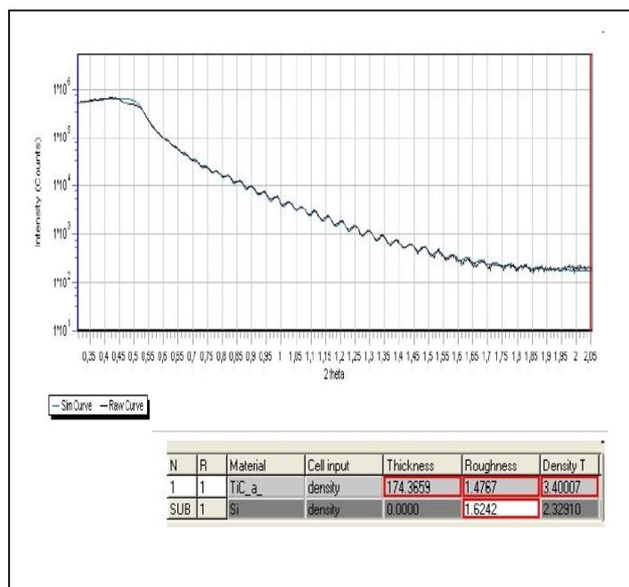
**Figure 8:** XRR measurement for a TiC film on silicon prepared at 200 W for 14 min. In this figure the y-axis is given as intensity in arbitrary units instead of the normalised reflectivity. The fit parameters for the simulation curve are highlighted in red. The parameter values are; layer thickness 174.37 nm, roughness 1.48 Å and density 3.40 g/cm<sup>3</sup>.
