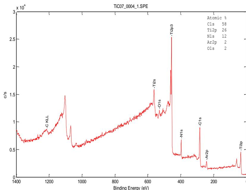
**Figure 14:** XPS survey spectrum of a 488 nm TiC film deposited on silicon at 200 W. This was obtained after sputter etching for 2 min. The atomic percentage of the elements are 58% C 1s, 26% Ti 2p, 12% N 1s, 2% O 1s, and 2% for Ar 2p.
