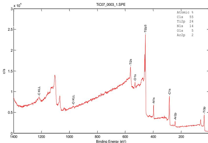
**Figure 13:** XPS survey spectrum of a 488 nm TiC film deposited on silicon at 200 W. This was obtained after sputter etching for 1 min. The atomic percentage of the elements are 55% C 1s, 24% Ti 2p, 14% N 1s, 5% O 1s, and 2% for Ar 2p.
