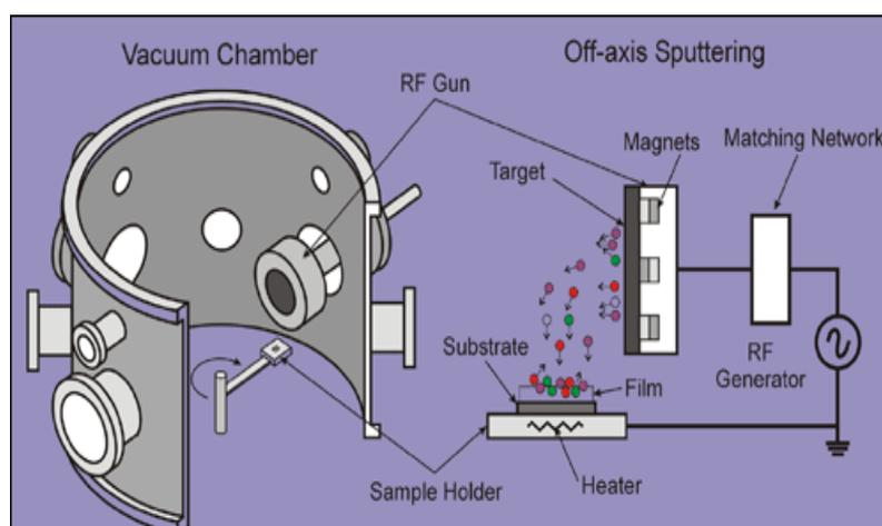
**Figure 2:** Schematic diagram of RF sputter system with the sputtering process shown adjacent thereto (after [www.phasis.ch](http://www.phasis.ch)).
