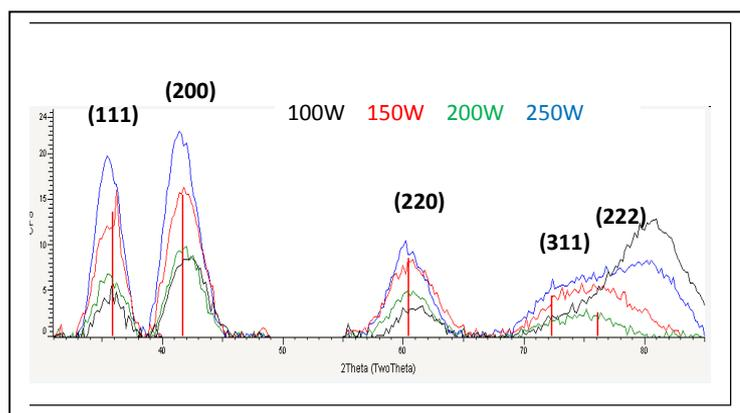
**Figure 10:** GIXRD measurements for TiC films prepared at 100 W, 150 W, 200 W and 250 W.
