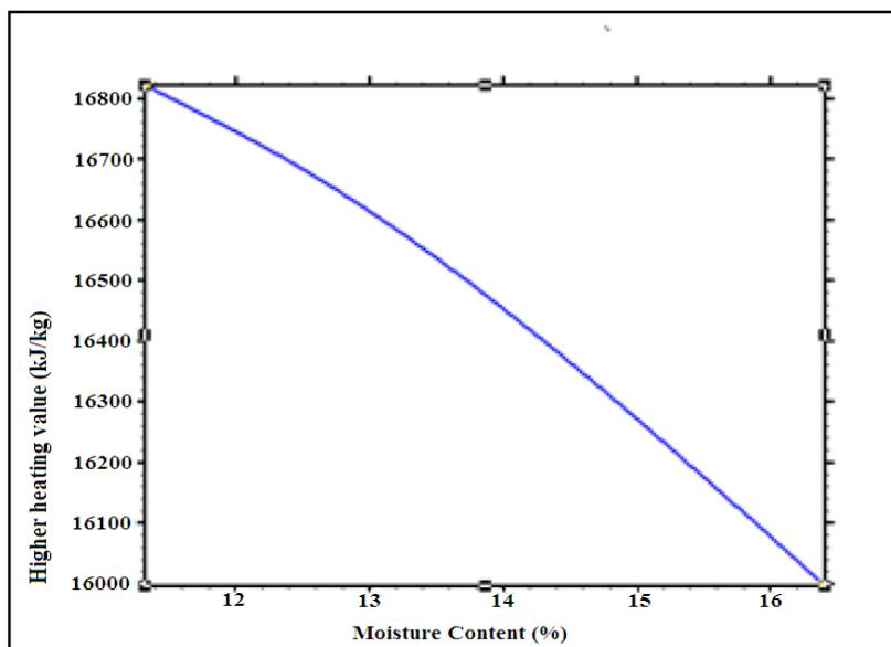
**Figure 7:** Heating values of samples as a function of moisture content.
