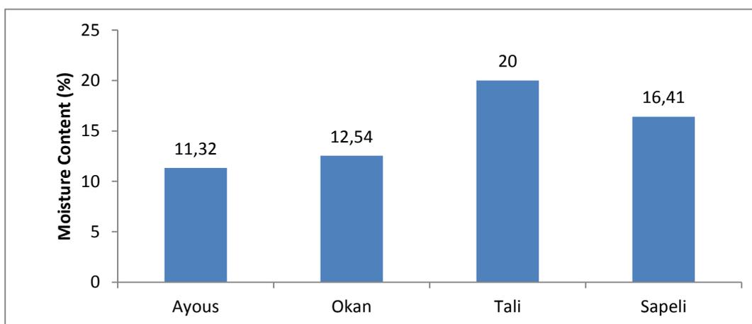
**Figure3:** moisture content of wood samples
