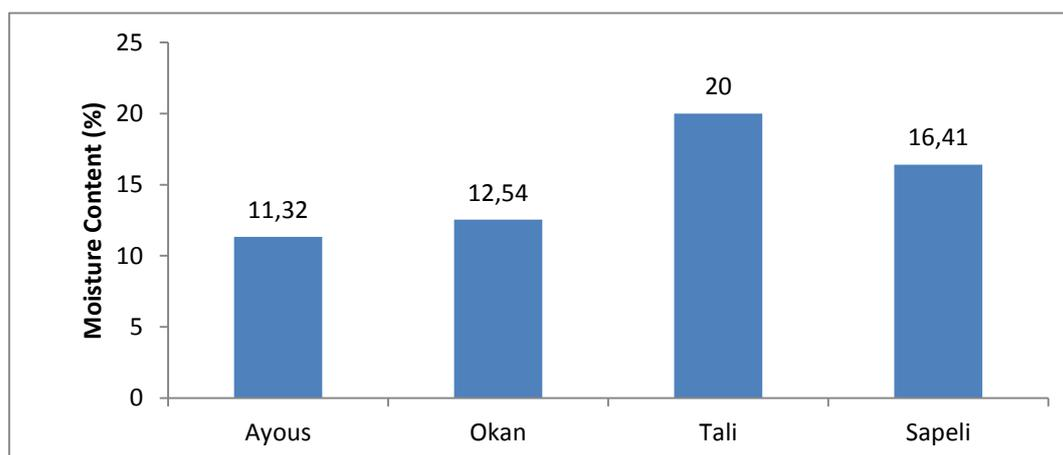
**Figure3:** moisture content of wood samples
