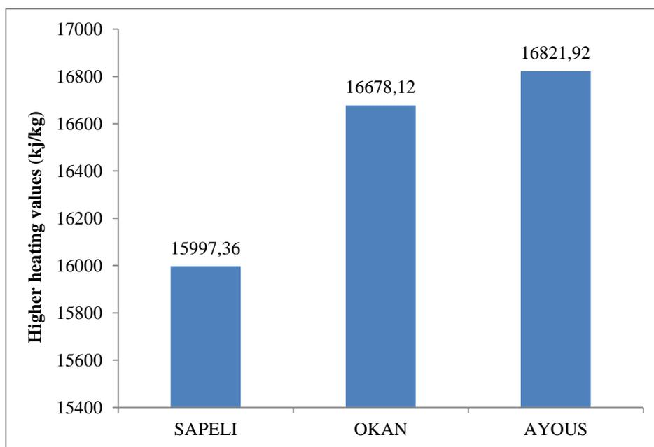
**Figure 6:** Higher heating values of some wood samples
