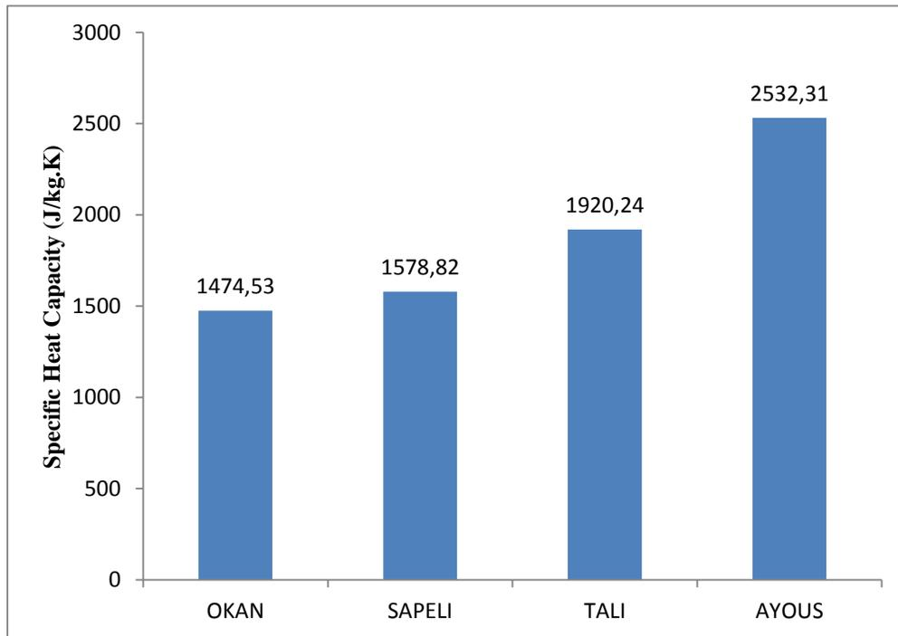
**Figure 5:** Specific heat capacity of each wood sample
