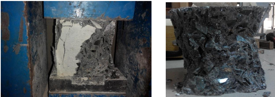
Figure 9: Crushed glass concrete cube at failure
