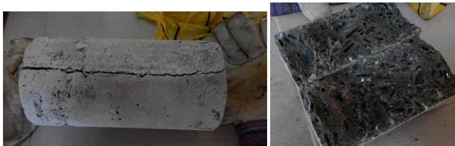
Figure 10: Failed pattern of glass concrete cylinder after testing
