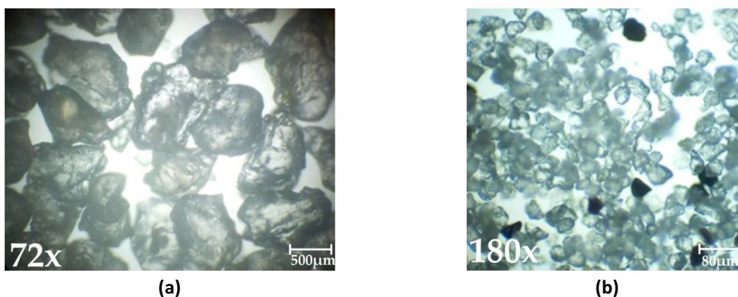
Figure 6: Micrograph of 500 microns (a) and 80 microns sand (b)
