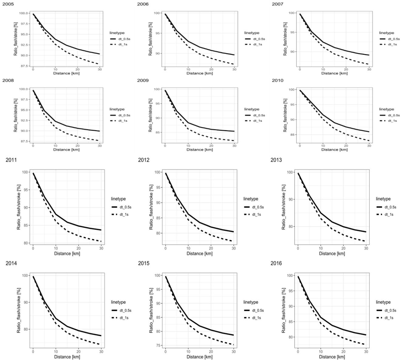
**Figure 3:** Ratio between the number of WWLLN flashes and that of strokes as a function of the distance criterion for two distinct time criteria.
