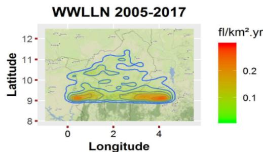
**Figure 11:** WWLLN flash density of the period data with a resolution of  $0.1^\circ \times 0.1^\circ$ .
