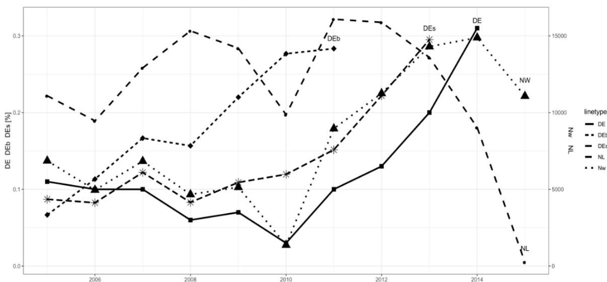
**Figure 4:** Annual number of flashes detected by WWLLN (Nw) and that by LIS (NL), and the estimated detection efficiency of WWLLN relative to the LIS (DE) and those found by [2] (DE<sub>b</sub>) and by [64] (DE<sub>s</sub>).
