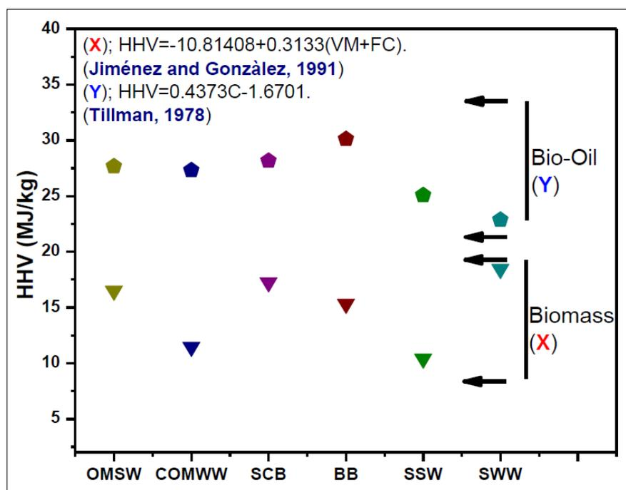
Figure 10: Higher heating value (HHV) of biomass and bio-oil.
