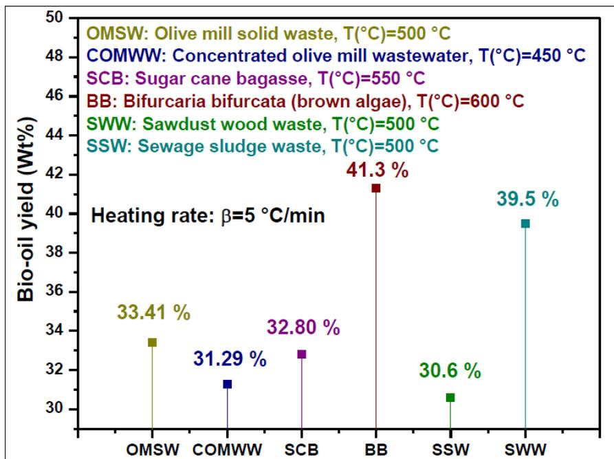
Figure 9: Optimal yield of bio-oil from pyrolysis.
