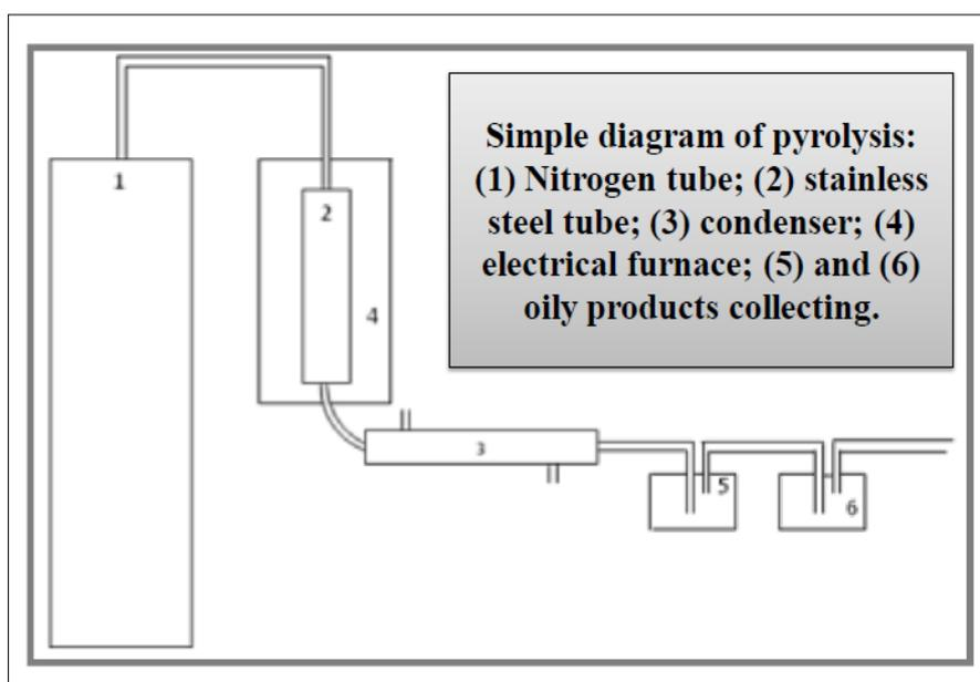
Figure 6: Simple diagram of pyrolysis.
