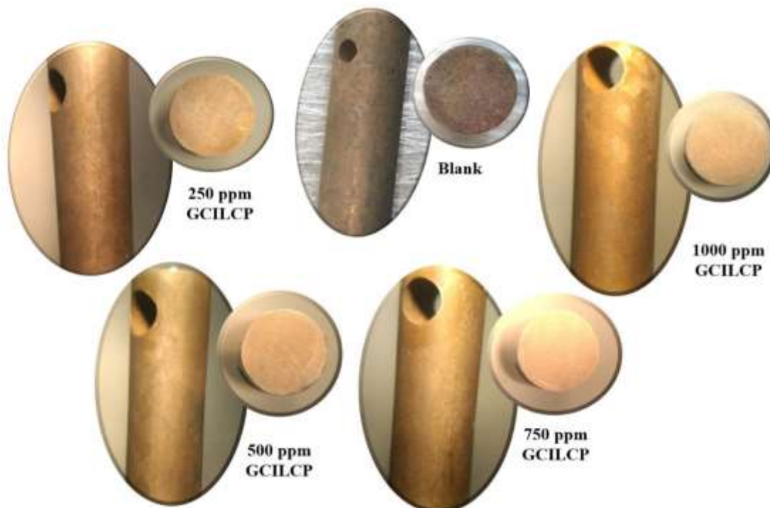
Figure 8. Corrosion inhibition efficiency of GCILCP on AISI 1018 carbon steel in 0.5 M H 2 SO 4 determined by weight loss in 6 h as immersion time at 25 ± 2 °C
