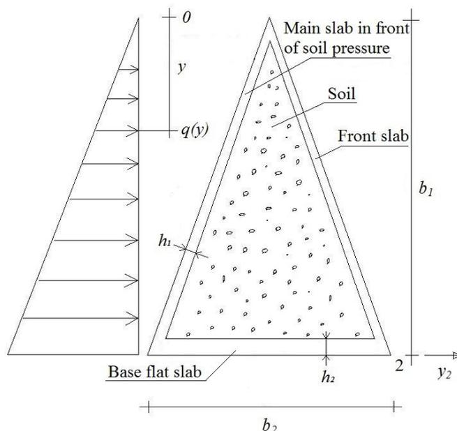
**Figure 1:** New retaining wall made of flat slabs.
