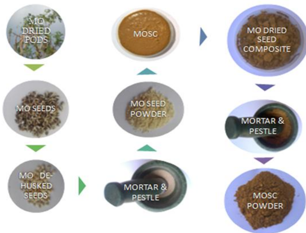
Fig. 2 Moringa oleifera seed composite preparation method
