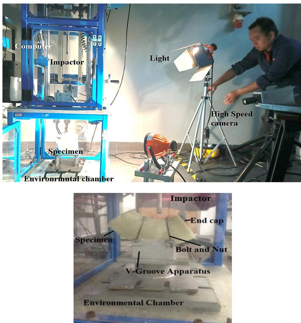
**Figure 4:** The setup of IMATEK Ltd drop impact testing machine and the test jig used for impact testing.
