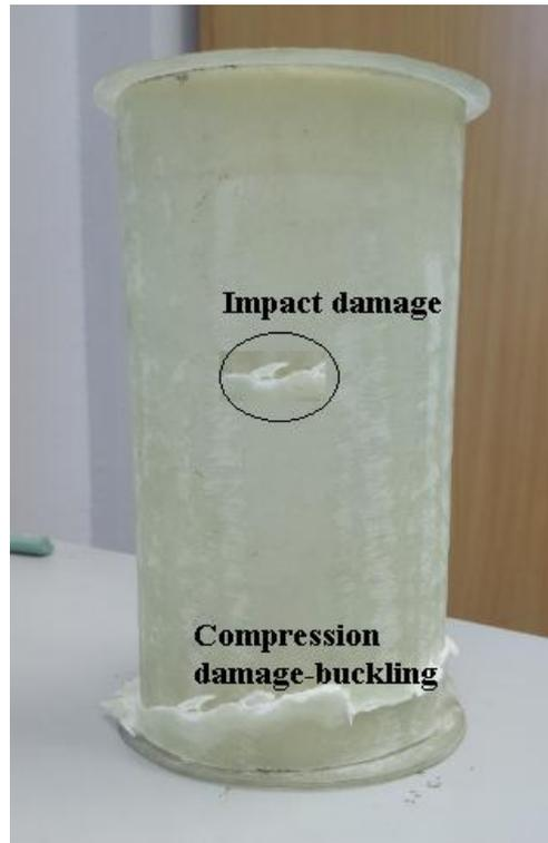
**Figure 15:** Compression damage and buckling damage in a sample E-glass fiber/epoxy composite pipe
