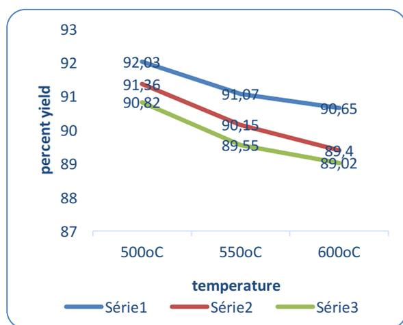
**FIG 1:** Temperature effect on yield of coconut shell ac
