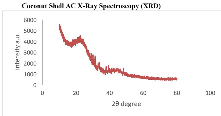
**Fig 7:** Coconut Shell X-Ray spectra.
