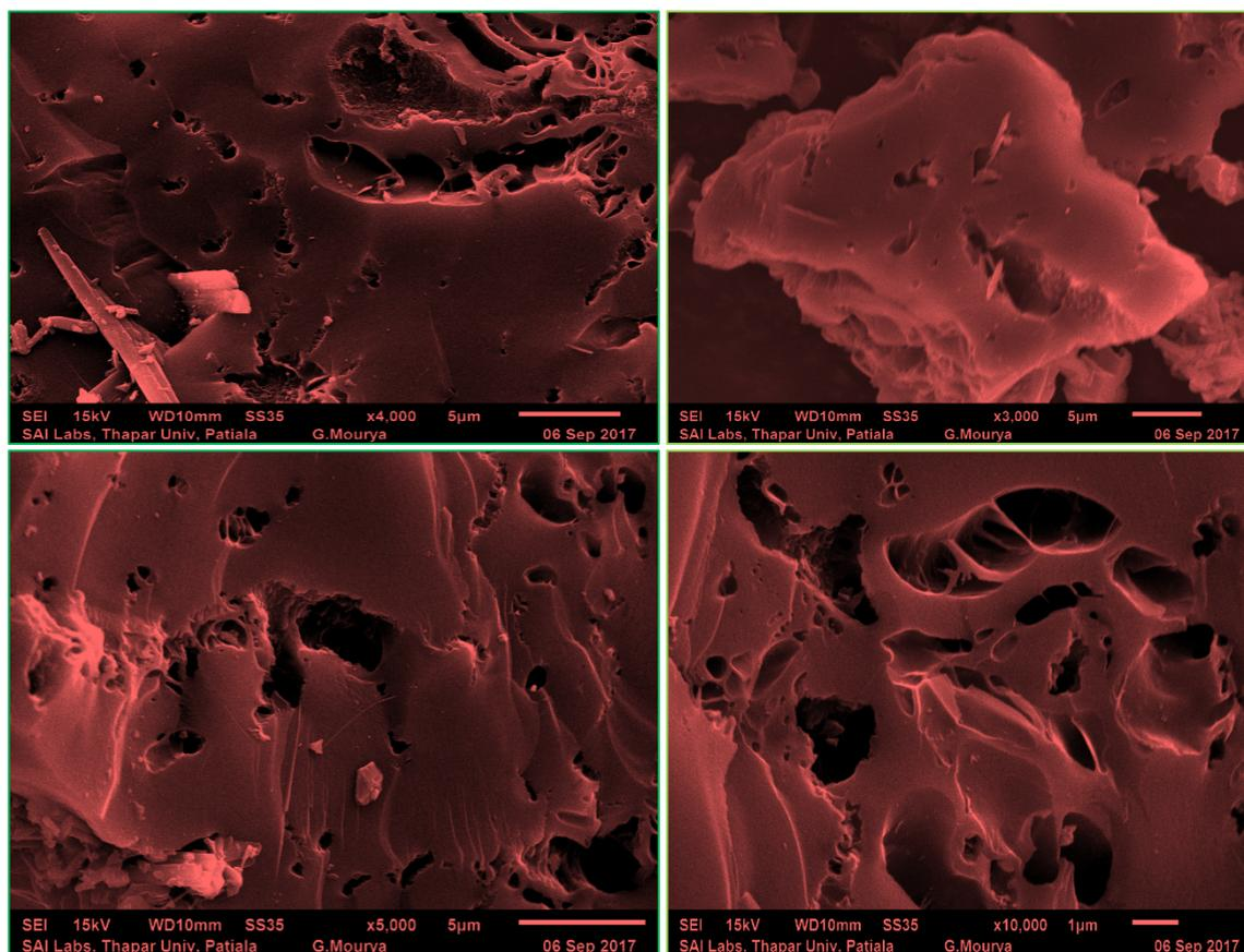
Fig 5: SEM images for Coconut Shell Activated Carbon at various magnification.
