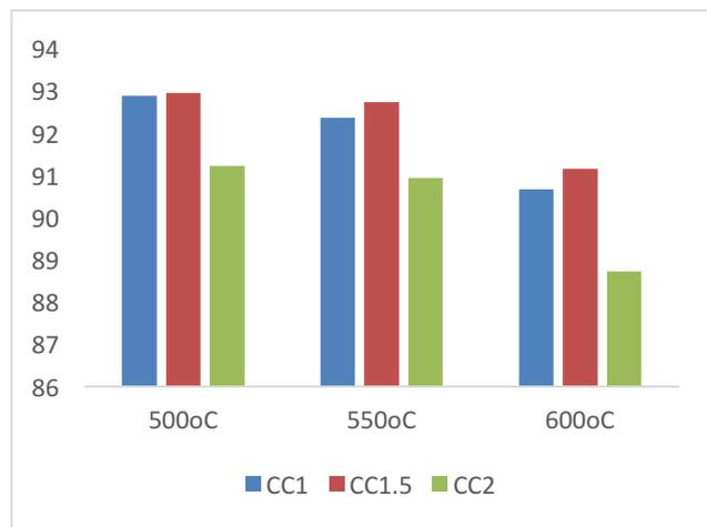
FIG 4: Impregnation ratio effect on yield of Corncob ac.
