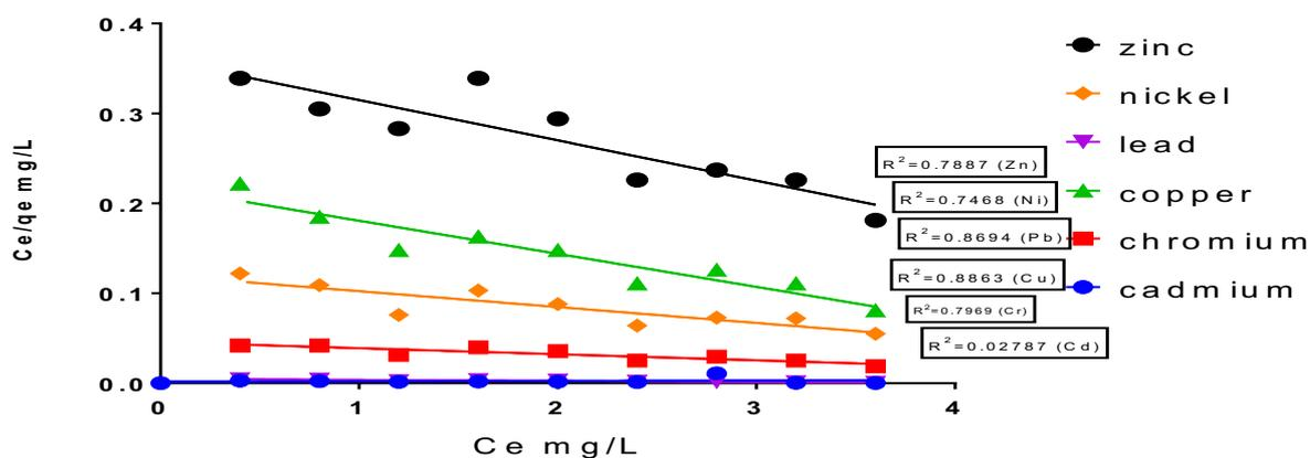
**Fig 9:** Coconut shell AC heavy metal adsorption.
