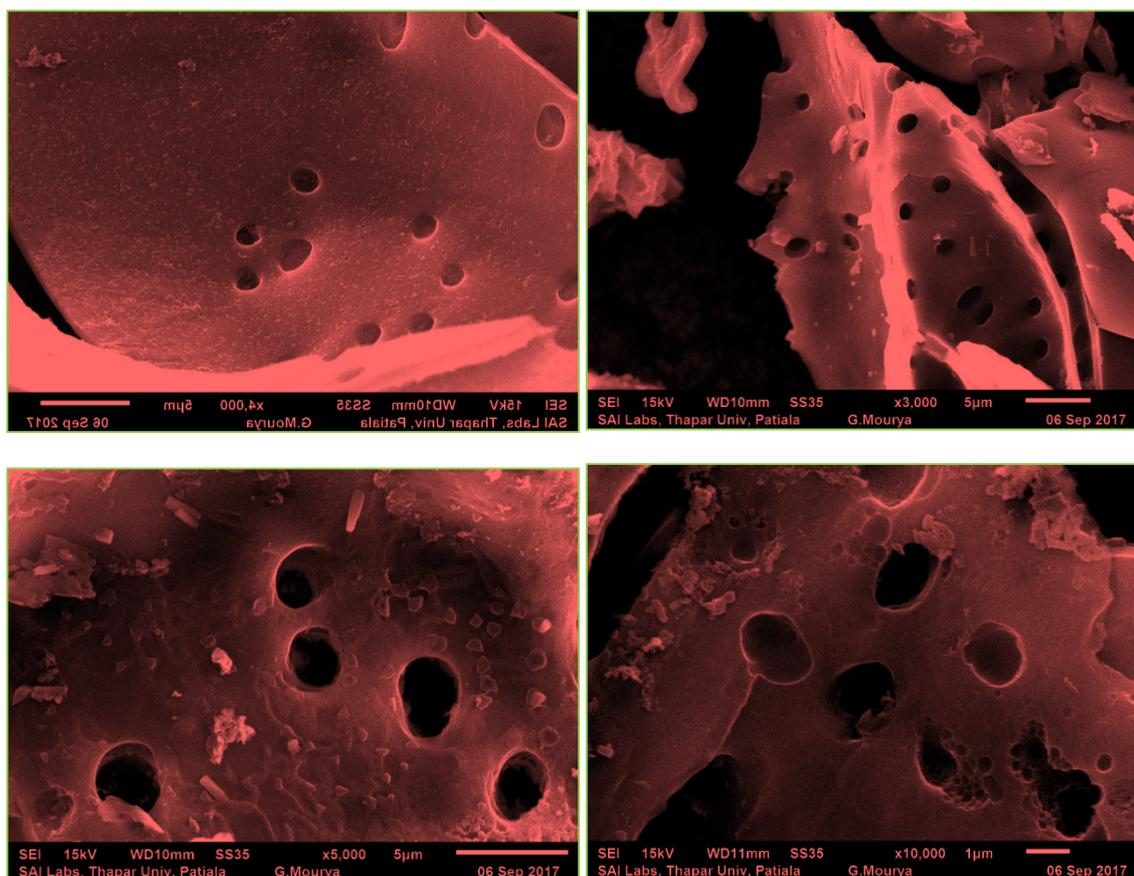
**Fig 6:** SEM images for Corncoobs Activated Carbon at various magnification.
