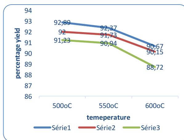
**FIG 2:** Temperature effect on yield of corncobs ac
