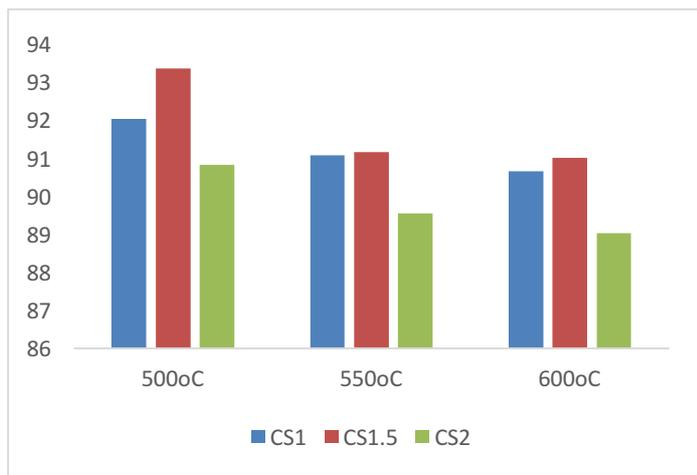
FIG 3: Impregnation ratio effect on yield of coconut Shell ac.
