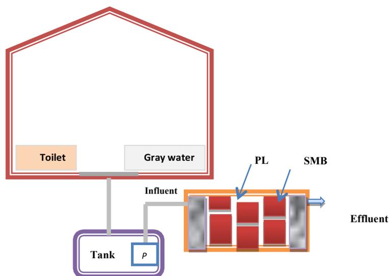
**Figure 1.** Schematic representation of Horizontal Multi-Soil-Layering (H-MSL) for a single household
