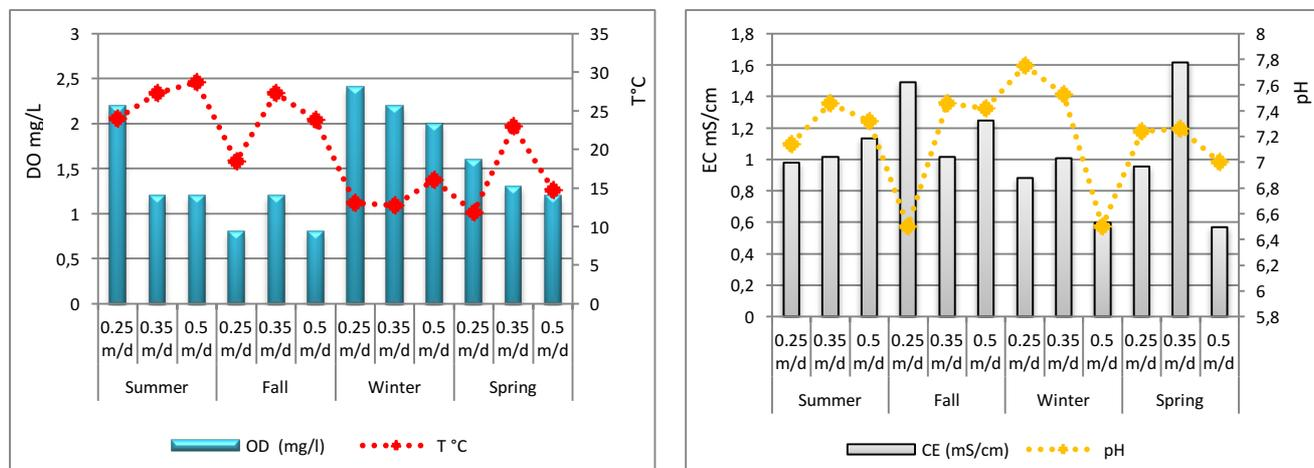
**Figure 2:** Trend of DO and temperature in H-MSL **Figure 3:** Trend of EC and pH in H-MSL
