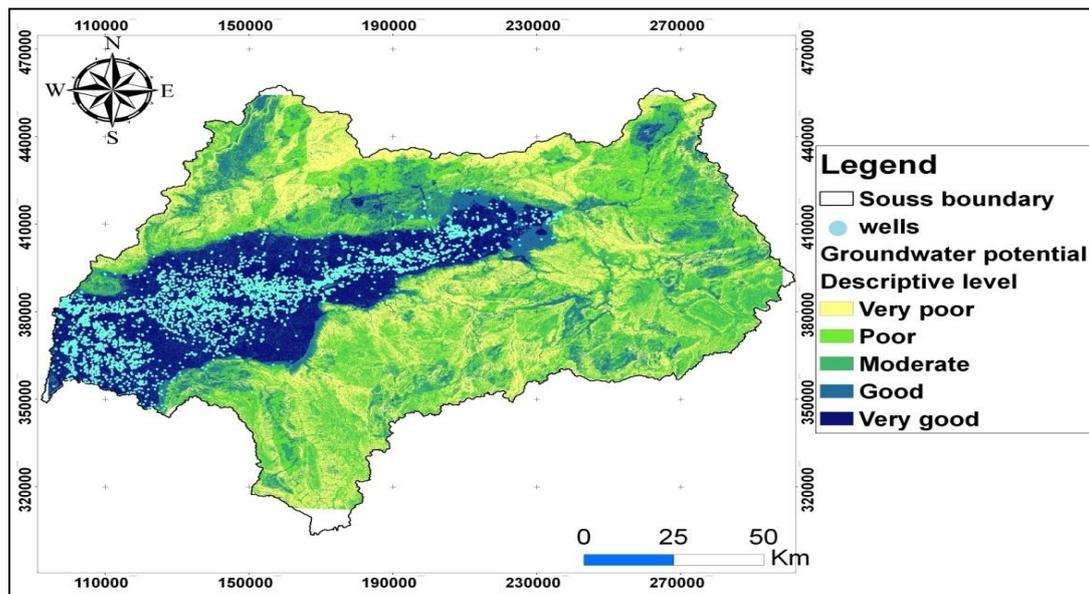
Figure 10 : Distribution of wells in groundwater potential zone map
