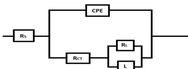
**Figure 5.** Equivalent circuit used to model EIS values of corrosion of AISI 1018 carbon steel in 0.5 M H<sub>2</sub>SO<sub>4</sub> without and with *Crataegus mexicana*.
