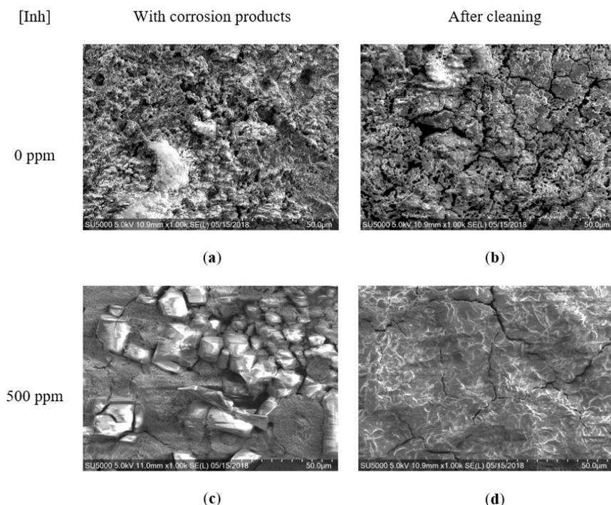
**Figure 8.** Micrographs of AISI 1018 carbon steel surface exposed to corrosion media without and with *Crataegus mexicana* as eco-friendly corrosion inhibitor.
