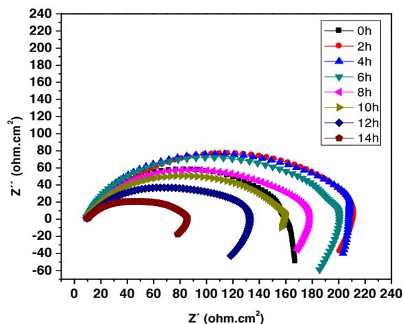
**Figure 6.** EIS of corrosion of AISI 1018 carbon steel in 0.5 M H<sub>2</sub>SO<sub>4</sub> with *Crataegus mexicana* at different residence times
