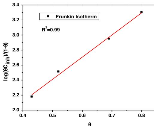
**Figure 7.** Frumkin adsorption isotherm from *Crataegus mexicana* eco-friendly corrosion inhibitor
