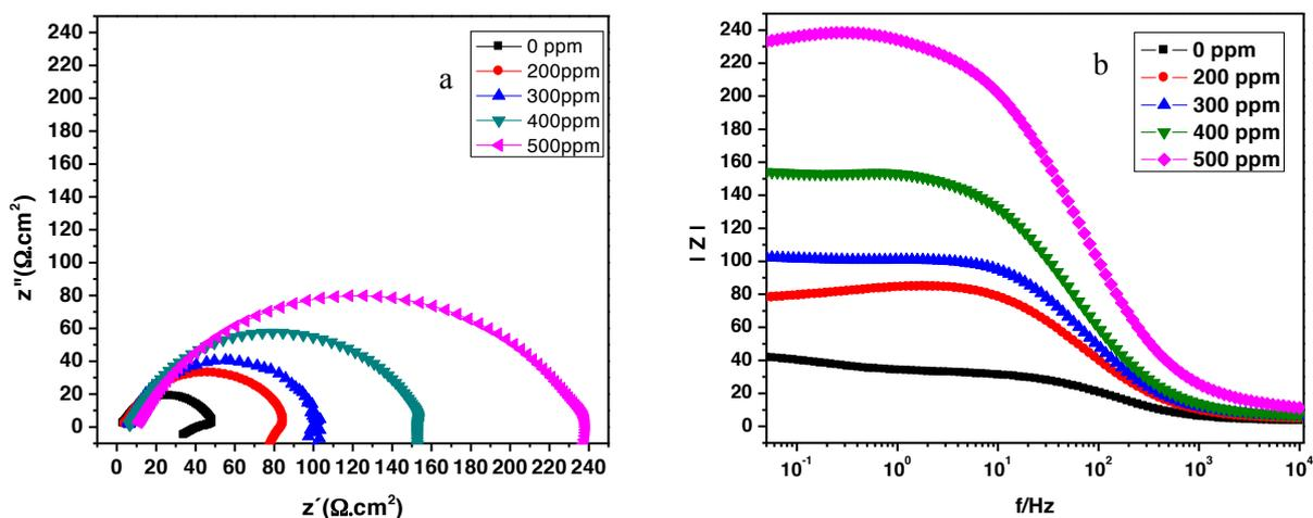
**Figure 4.** EIS of corrosion of AISI 1018 carbon steel in 0.5 M H<sub>2</sub>SO<sub>4</sub> without and with *Crataegus mexicana* a) Nyquist diagram b) Bode diagram.
