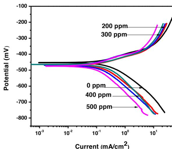
**Figure 3.** PPC of corrosion of AISI 1018 carbon steel in 0.5 M H<sub>2</sub>SO<sub>4</sub> without and with *Crataegus mexicana*.
