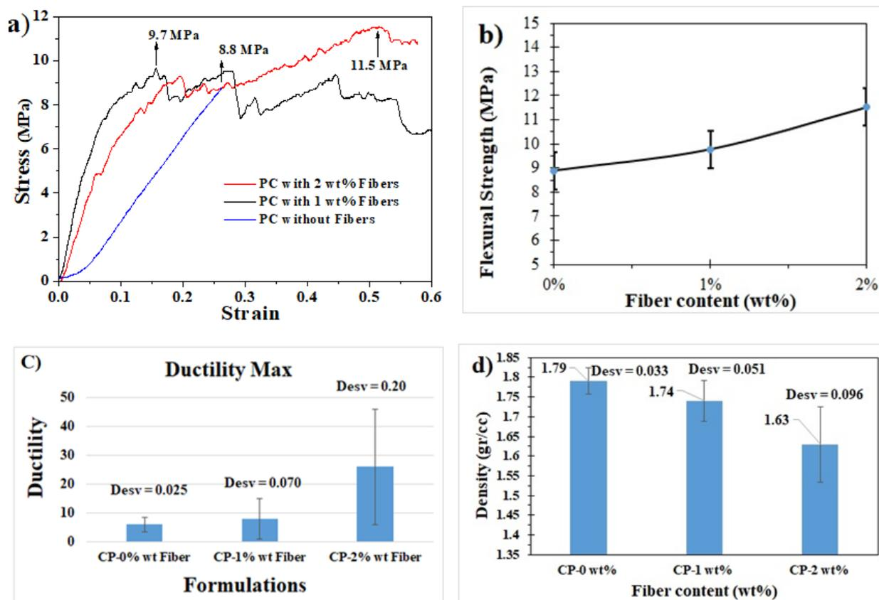
**Figure 2:** Flexural strength and density results for samples: a) typical strain-stress curves, b) flexural strength mean values, c) ductility, d) density.
