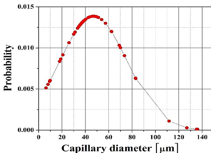
**Figure 4:** Pore (capillarity) diameter distribution for the fibers.
