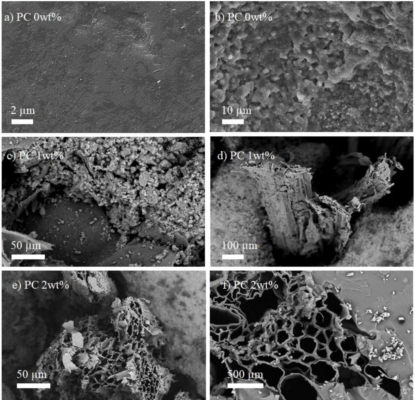
**Figure 5:** SEM images of cement paste reinforced with sugar cane fibers
