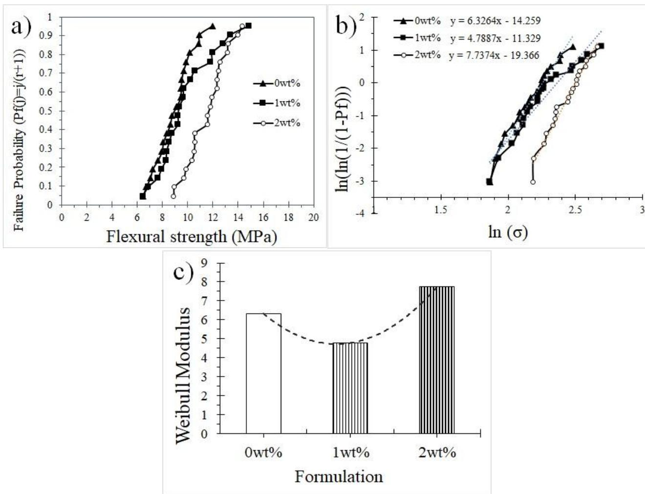
Figure 6: Weibull distribution results for the different samples
