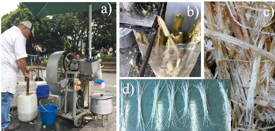
**Figure 1:** Extraction of fibers from sugarcane bagasse, a) machine used for the juice extraction from sugarcane for beverage; b) raw sugarcane for the machine; c) detail of the bagasse; d) selected and cleaned fibers from c).
