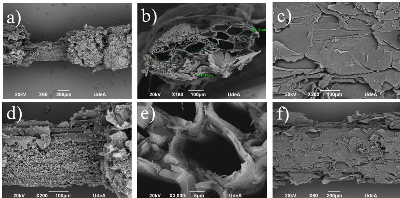
**Figure 3:** SEM images of sugarcane bagasse fibers after the cleaning process.
