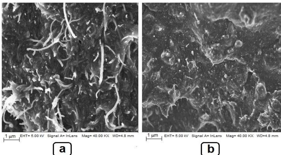
**Figure 2:** FESEM images of (a) BCNTPE (b) SDSMCNTPE.
