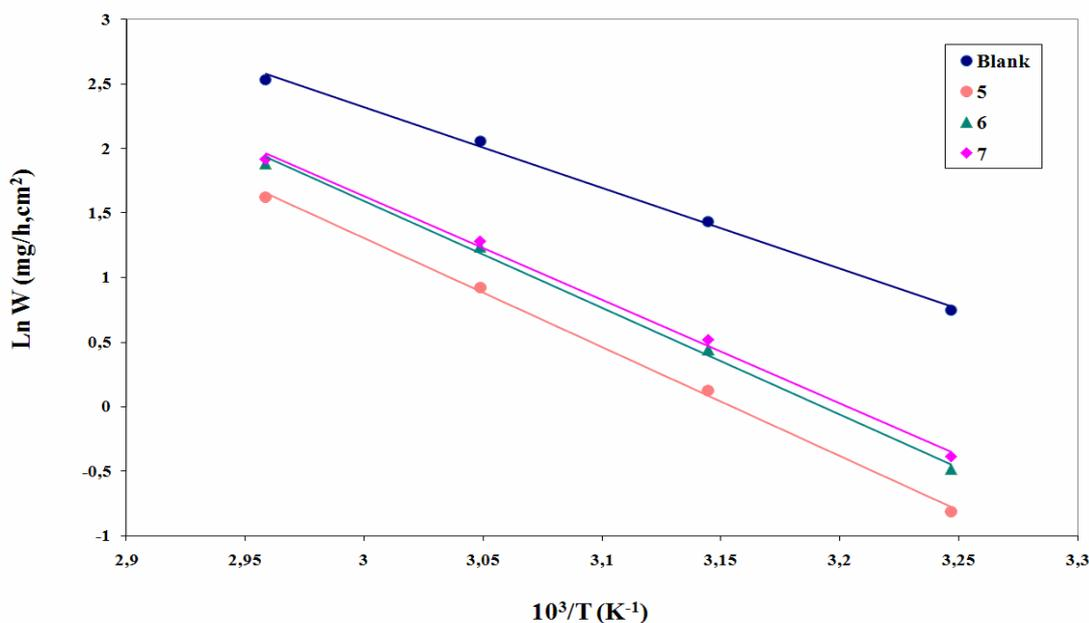
**Figure 1:** Arrhenius plots of steel in uninhibited and inhibited acid
