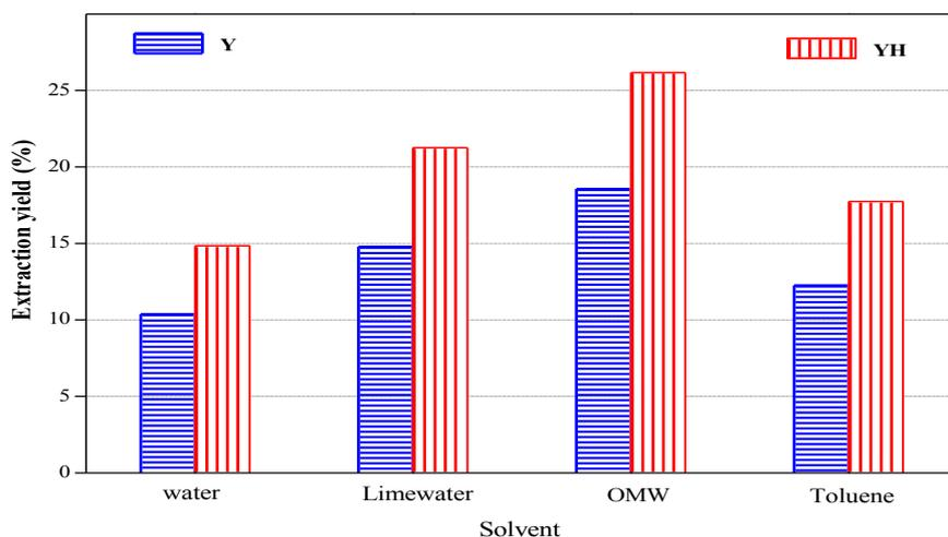
**Figure 5:** Effect of mineral matrix and solvent on extraction yield
