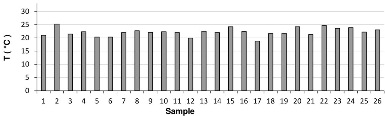
**Figure 4:** Variation of the groundwater temperature of the Barremo-Aptian aquifer in Essaouira basin (2015 companion)
