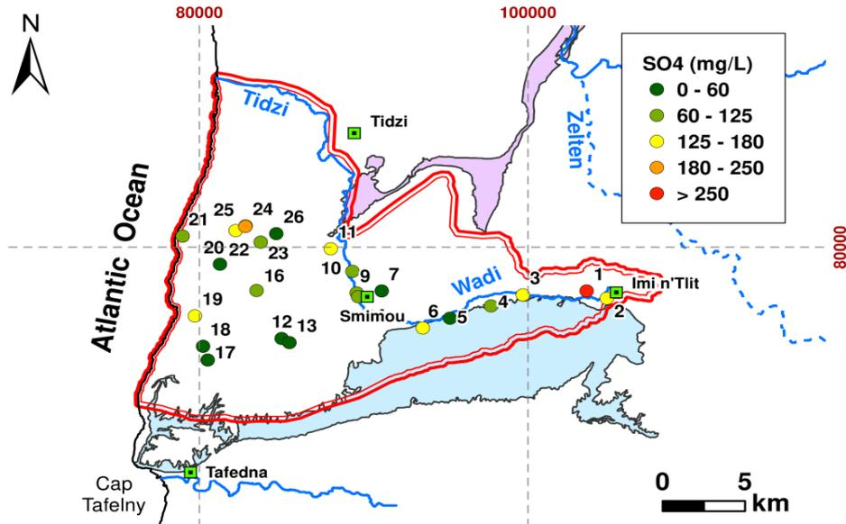
**Figure 10:** Spatial distribution of groundwater sulfates in the Barremo-Aptian aquifer of Essaoira basin (2015 companion)
