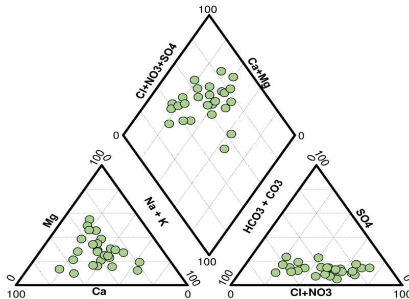
**Figure 7:** Piper diagram of groundwater from the Barremo-Aptian aquifer within Essauira basin (2015 companion)
