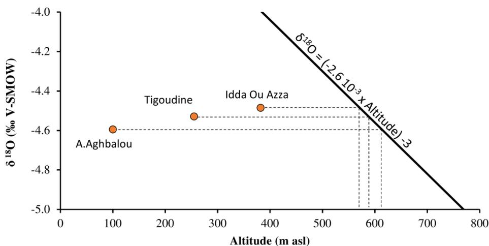
**Figure 18:** Determination of the average recharge altitudes of the Barremo-Aptian aquifer in Essauira basin using Oxygen-18 contents
