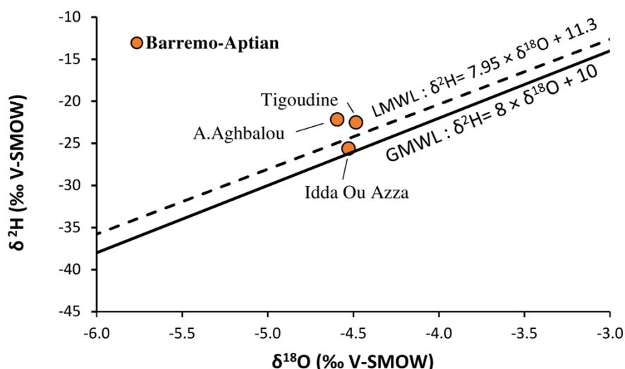
**Figure 17:**  $^2\text{H}$ - $^{18}\text{O}$  correlation diagram of the groundwater of the Barremo-Aptian aquifer from Essauira basin
