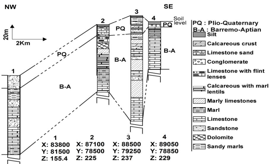
Figure 2: Lithological sections of the wells catching the Barremo-Aptian aquifer [13] (modified)
