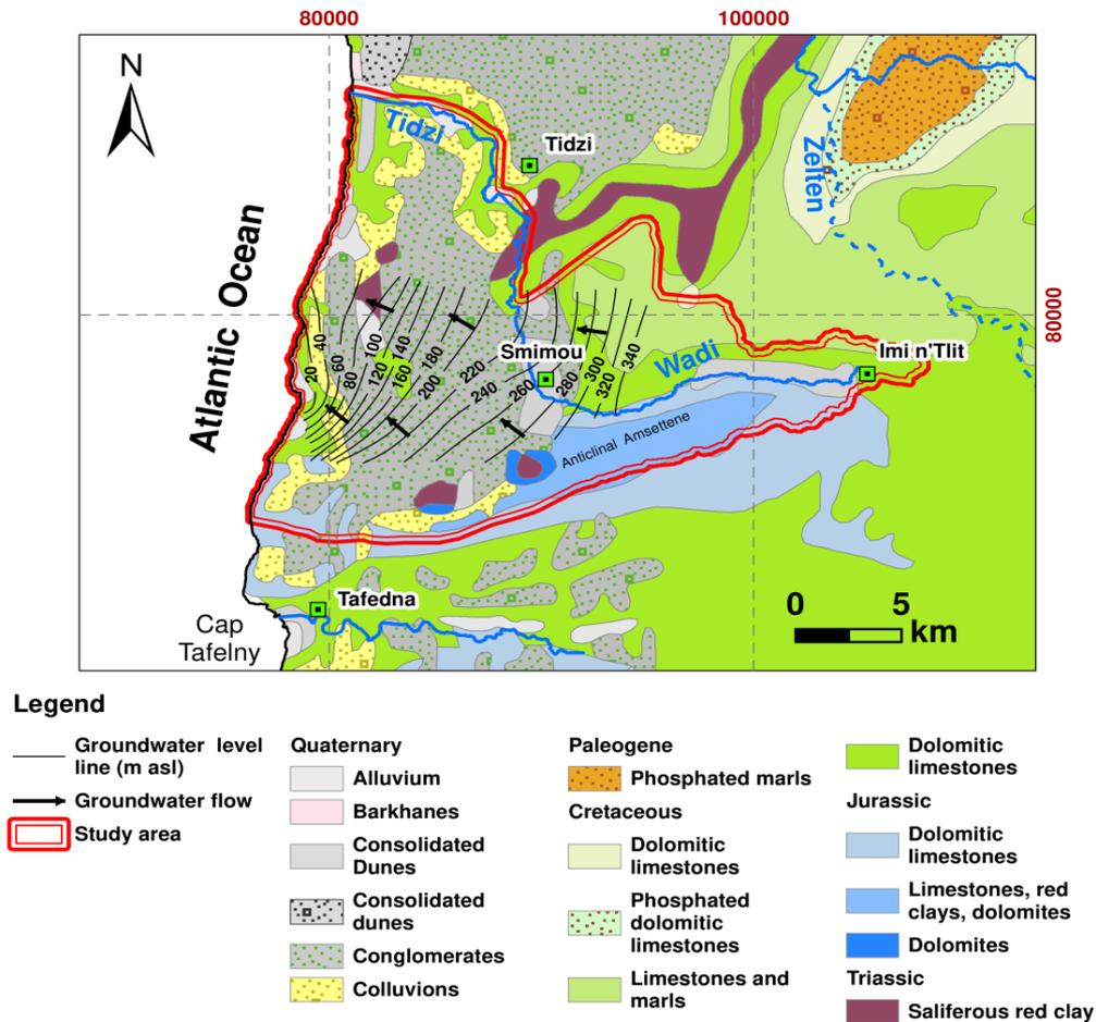
**Figure 3:** Geological and Piezometric map (June 2015) of the Study Area [14] (modified)
