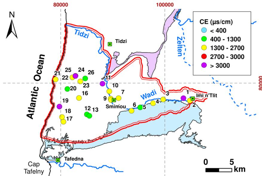
**Figure 6:** Spatial distribution of the groundwater electrical conductivity of the Barremo-Aptian aquifer in Essauira basin (2015 companion)
