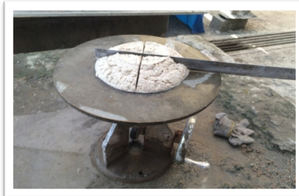
Figure 7. The diameter of the lime mortar was measured to determine the workability
