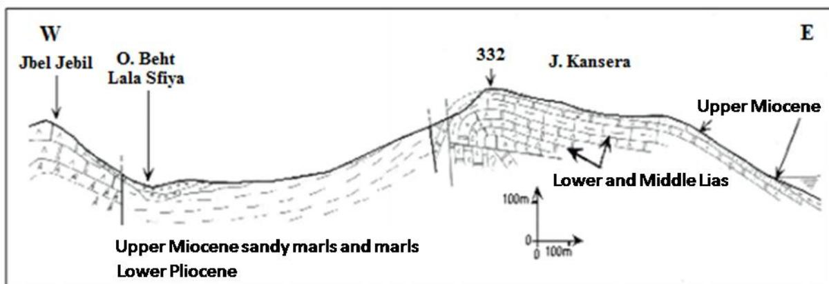
Figure 5: Geological cross-section of Jbel El Kansera [15].
