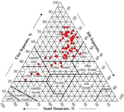
Figure 7: Distribution of clay, sand and silt in the soil samples
