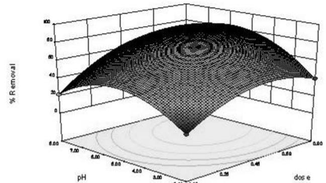
**Figure 7:** Effect of the interaction between adsorbent dose and pH on copper (II) removal.
