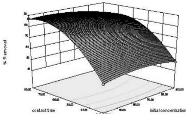
**Figure 6:** Effect of the interaction between initial concentration and contact time on copper (II) removal.
