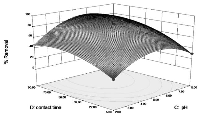
**Figure 9:** Effect of the interaction between pH and contact time on copper (II) removal.
