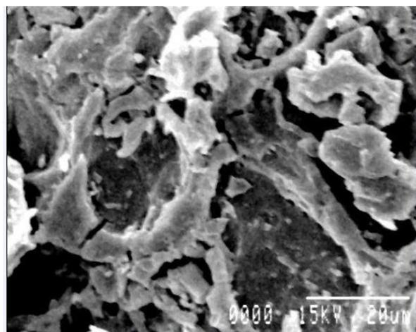
**Figure 3:** SEM image of NBP after treatment with copper (II).
