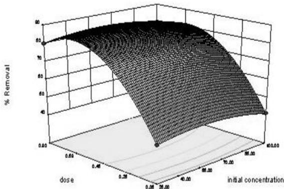
**Figure 4:** Effect of the interaction between adsorbent dose and initial concentration on copper (II) removal.
