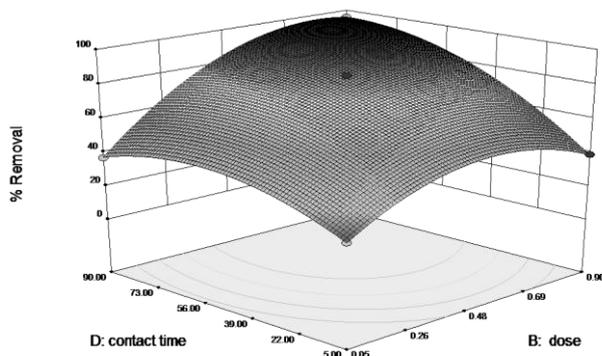
**Figure 8:** Effect of the interaction between contact time and adsorbent dose on copper (II) removal.
