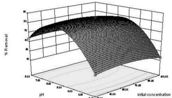
**Figure 5:** Effect of the interaction between pH and initial concentration on copper (II) removal.
