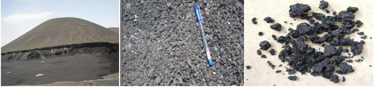
Figure 1: Deposit of Difan-Amran-Yemen extraction of the natural Pozzolan
