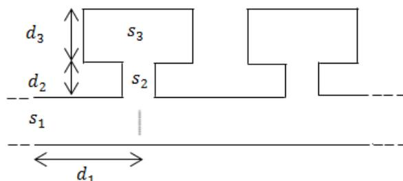
**Figure 1** Periodic structure with branched simple Helmholtz Resonator
