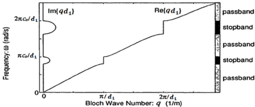
**Figure 4:** Illustration of stop-band and pass-band in general periodic structure [10]
