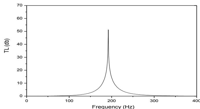
**Figure 6:** TL Coefficient corresponding to one cell ( $d_1=0.5\text{ m}$ ,  $d_2=0.1\text{m}$  and  $d_3=0.3\text{m}$ )
