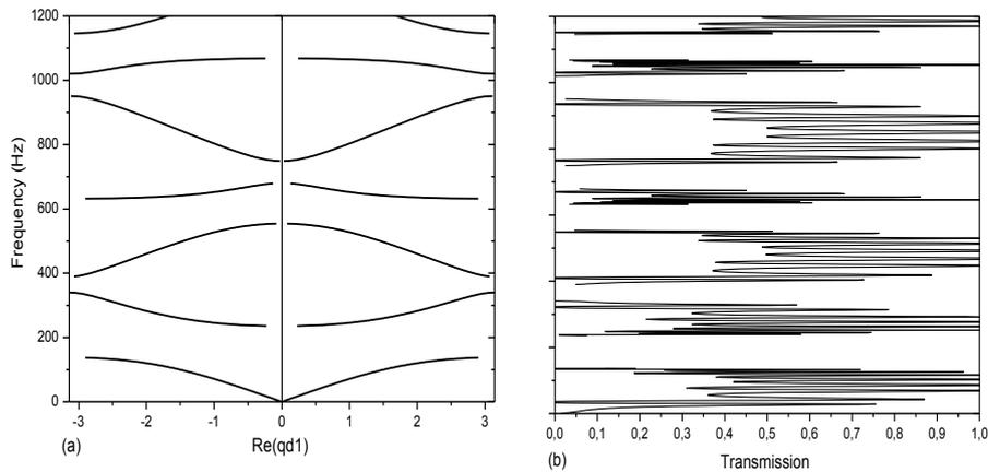
**Figure 5:** (a) Band structures and (b) Transmission  $T$  of a periodic system of 10 cells ( $N_c=10$ ) and for  $d_1=0.5\text{m}$ ,  $d_2=0.1\text{m}$  and  $d_3=0.3\text{m}$
