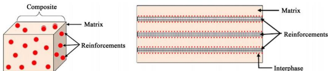
**Figure 1** Composition of laminate and inter-phase which include resin as a matrix and fiber as reinforcement
