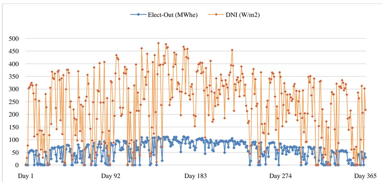
**Figure 3:** The daily electrical output and the DNI measurements.
