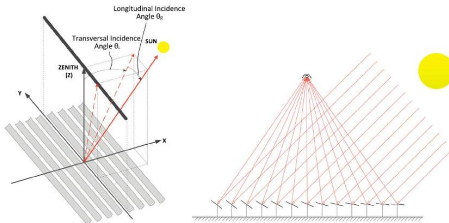
**Figure 1:** Schematic view of the incidence angles [20].
