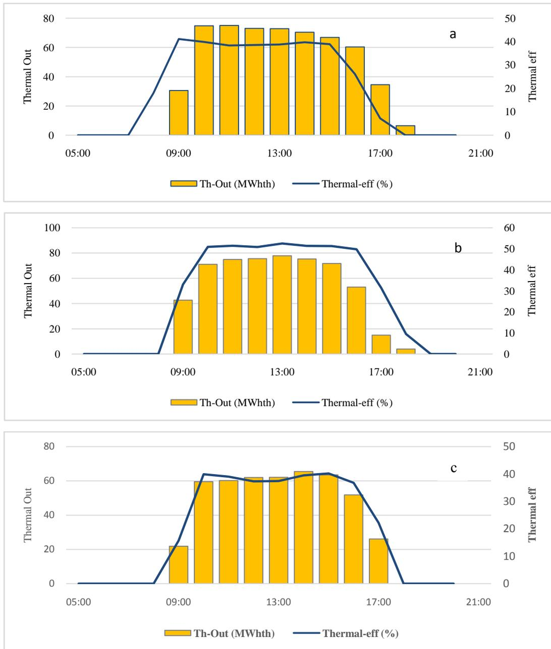
**Figure 6:** The hourly thermal output and thermal efficiency of the 10MW plant during the equinoxes. (a) The 21<sup>th</sup> of Marsh. (b) The 21<sup>th</sup> of June. (c) The 21<sup>th</sup> of September.
