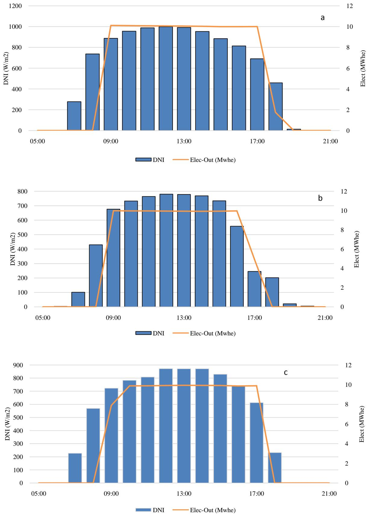
**Figure 5:** The hourly DNI and electrical output during the equinoxes. (a) The 21<sup>th</sup> of Marsh.(b) The 21<sup>th</sup> of June. (c) The 21<sup>th</sup> of September.
