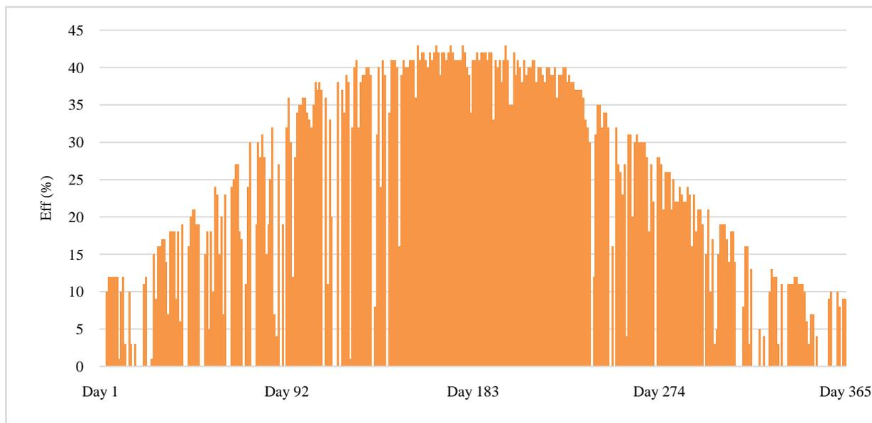
**Figure 4:** The daily thermal efficiencies of the 10MWe pilot.
