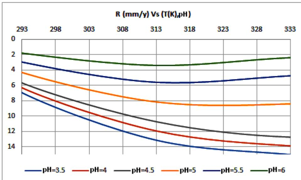
**Figure 3:** Effect of variation of hydrogen potential from standard medium (pH=6) to acid (pH=3.5) at low value of CO<sub>2</sub> % for temperatures range 293K to 333K
