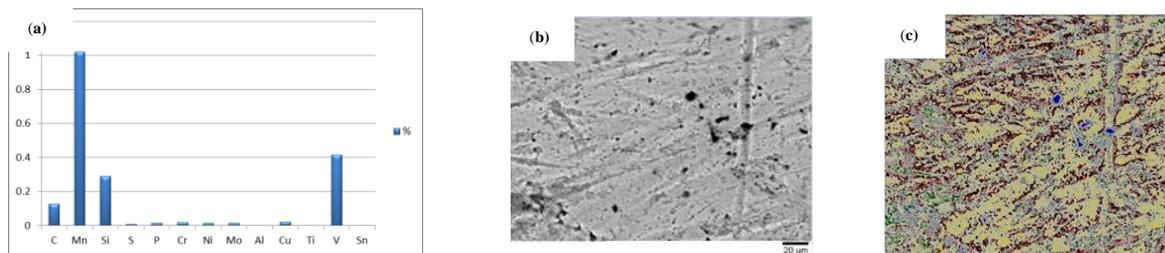
**Figure 1:** (a) : chemical composition of HLE steel; SEM fractographs of Steel (b): map 20um, (c): map 20um
