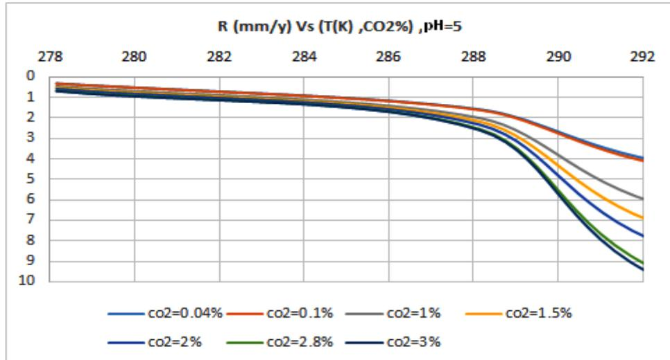
Figure 6: Effect of variation of CO<sub>2</sub>% and temperatures at pH=5 for temperature range of 278K-292K.
