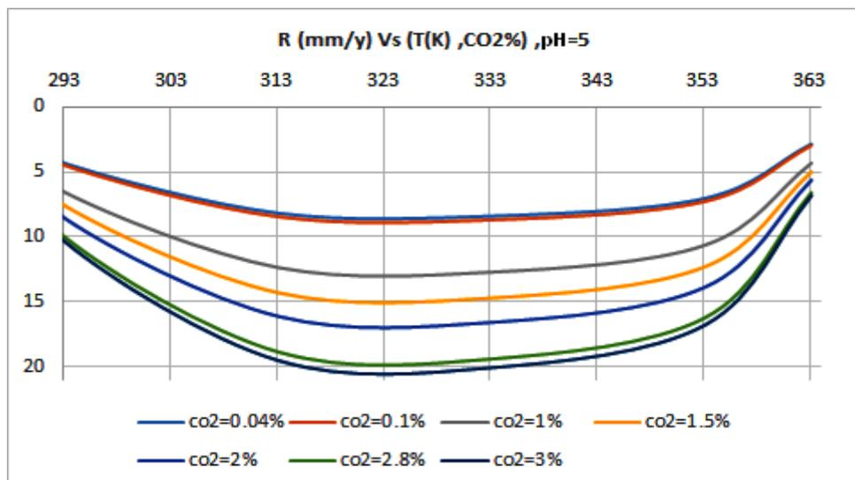
Figure 7: Effect of variation of CO<sub>2</sub> % and temperatures at pH=5 from 293K to 373K.
