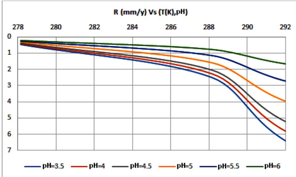
**Figure 2:** Effect of variation of hydrogen potential from standard medium (pH=6) to acid (pH=3.5) at low value of CO<sub>2</sub> % for temperature range 278K-292K.
