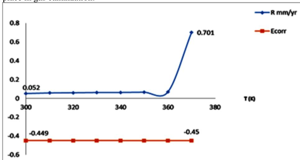
**Figure 8:** Corrosion rate vs temperature (NaCl medium) [1]
