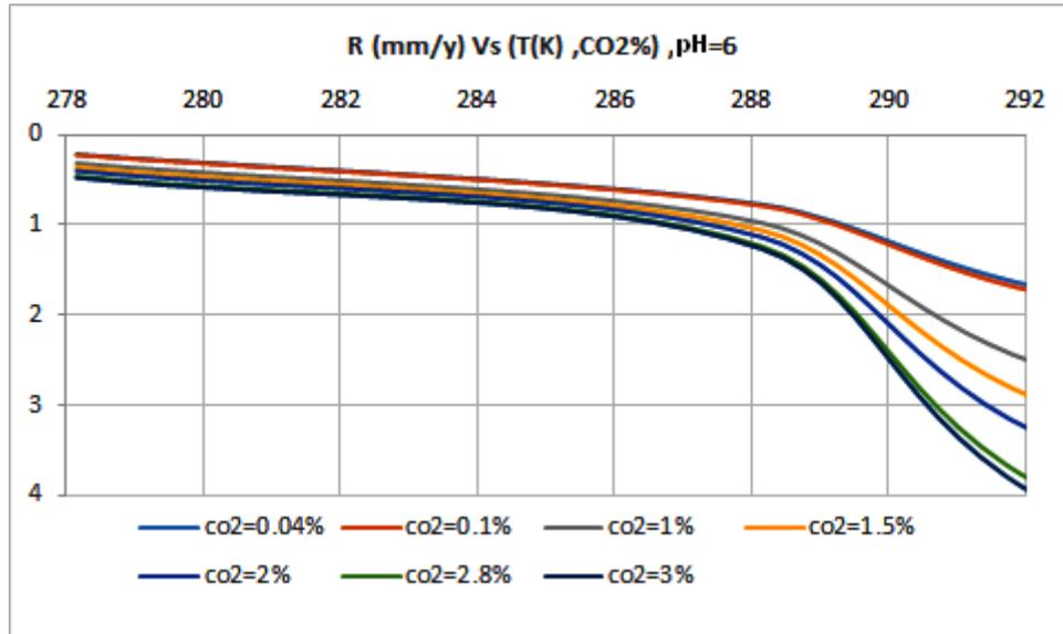
**Figure 4:** Effect of variation of CO<sub>2</sub>% and temperatures at pH=6 for temperature range 278K-292K.
