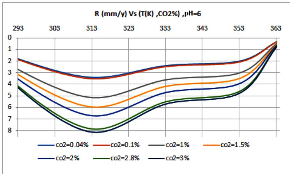
**Figure 5:** Effect of variation of CO<sub>2</sub>% and temperatures at pH=6 for temperature range 293K-363K.
