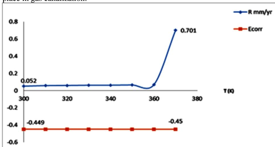
Figure 8: Corrosion rate vs temperature (NaCl medium) [1]
