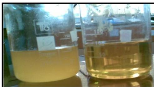
**Figure 1:** Waste cooking oil before (left) and after (right) treatment
