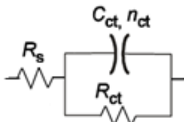
Figure 8: Equivalent circuit model for system Steel / 5 M HCl /mixture.
