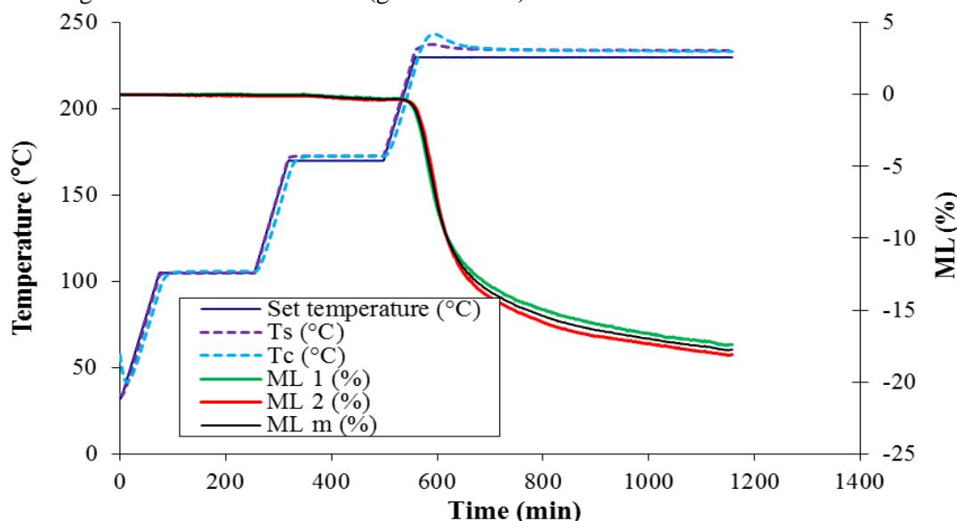
**Figure 2:** Thermo-degradation of beech wood treated at 230°C ( $1^{\circ}\text{C}.\text{min}^{-1}$ )
