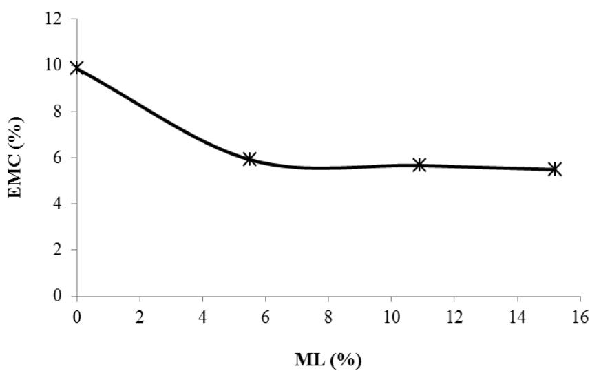
**Figure 4:** Relationship between mass loss (ML) due to thermal degradation of beech wood at 230°C and EMC
