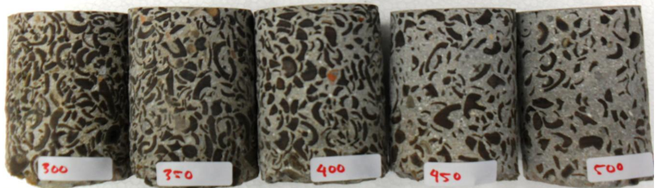
Figure 1: Distribution of OPS in concrete and cement content volume (left to right: 300,350,400,450 and 500 kg/m 3 cement content)
