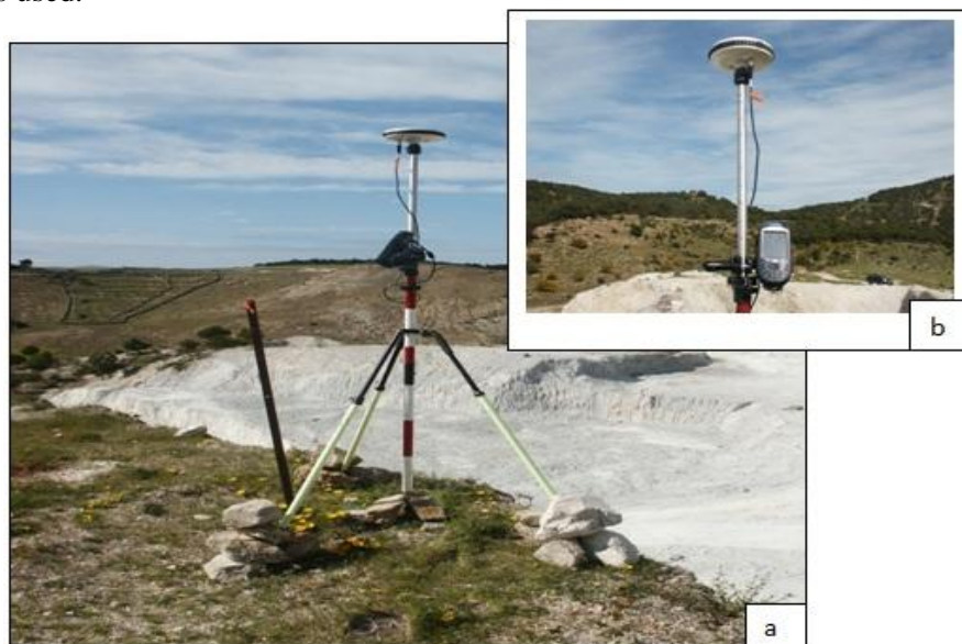
Figure 4: Station Ashtech ProMark2 GPS, a; Base tripod, b; close-up view
