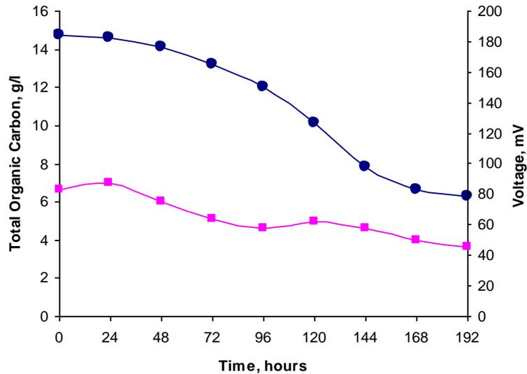
Fig. 2. Total Organic Carbon (●) and Voltage (■) vs. Time observed in the experiments with MFC
