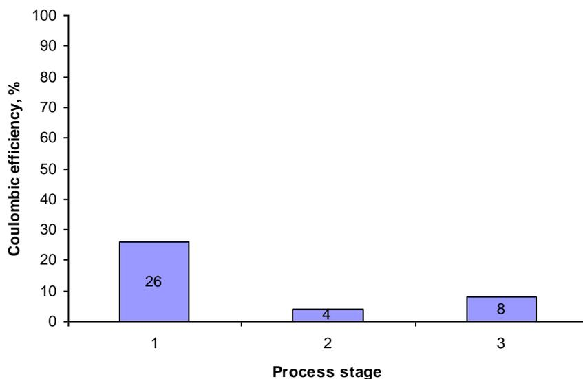
Fig. 3. Coulombic efficiency of the MFC during the different stages of the process (1<sup>st</sup> stage – 0 – 48h; 2<sup>nd</sup> stage 48-168h; 3<sup>rd</sup> stage 168-196h)
