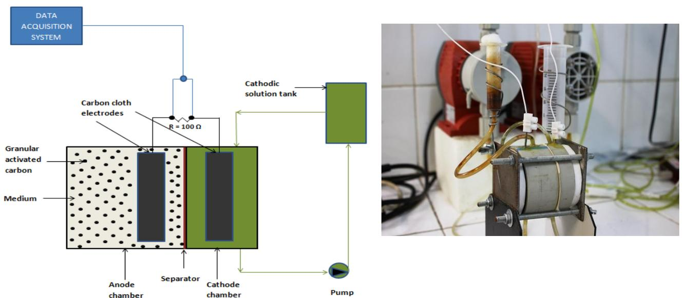
Fig. 1. Design of the Microbial Fuel Cell (left) and real reactor (right) used in this study
