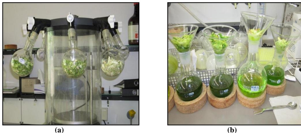
**Figure 3:** scheme of all samples frozen at  $-80^{\circ}\text{C}$  and lyophilized over night to reduce water content in the samples (a) preparing them for extraction with organic solvents (b).
