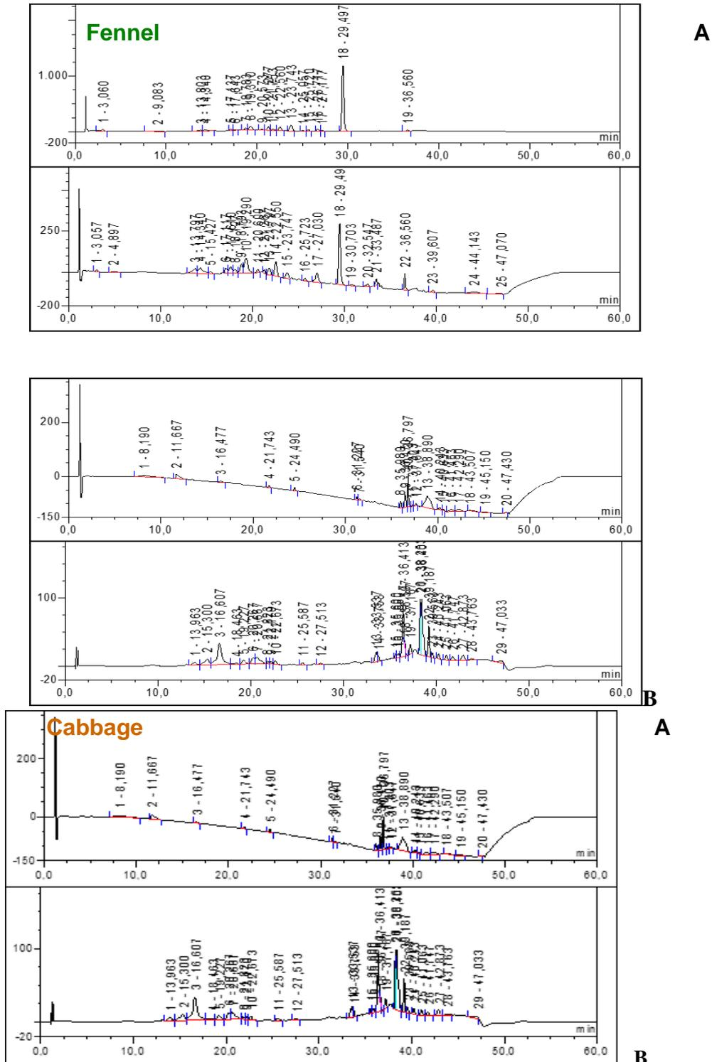
**Figure 4:** UHPLC analysis of vegetable Samples; **A:** Blank vegetable samples without pesticide treatment **B:** Samples treated with an illegal dose of cypermethrin.
