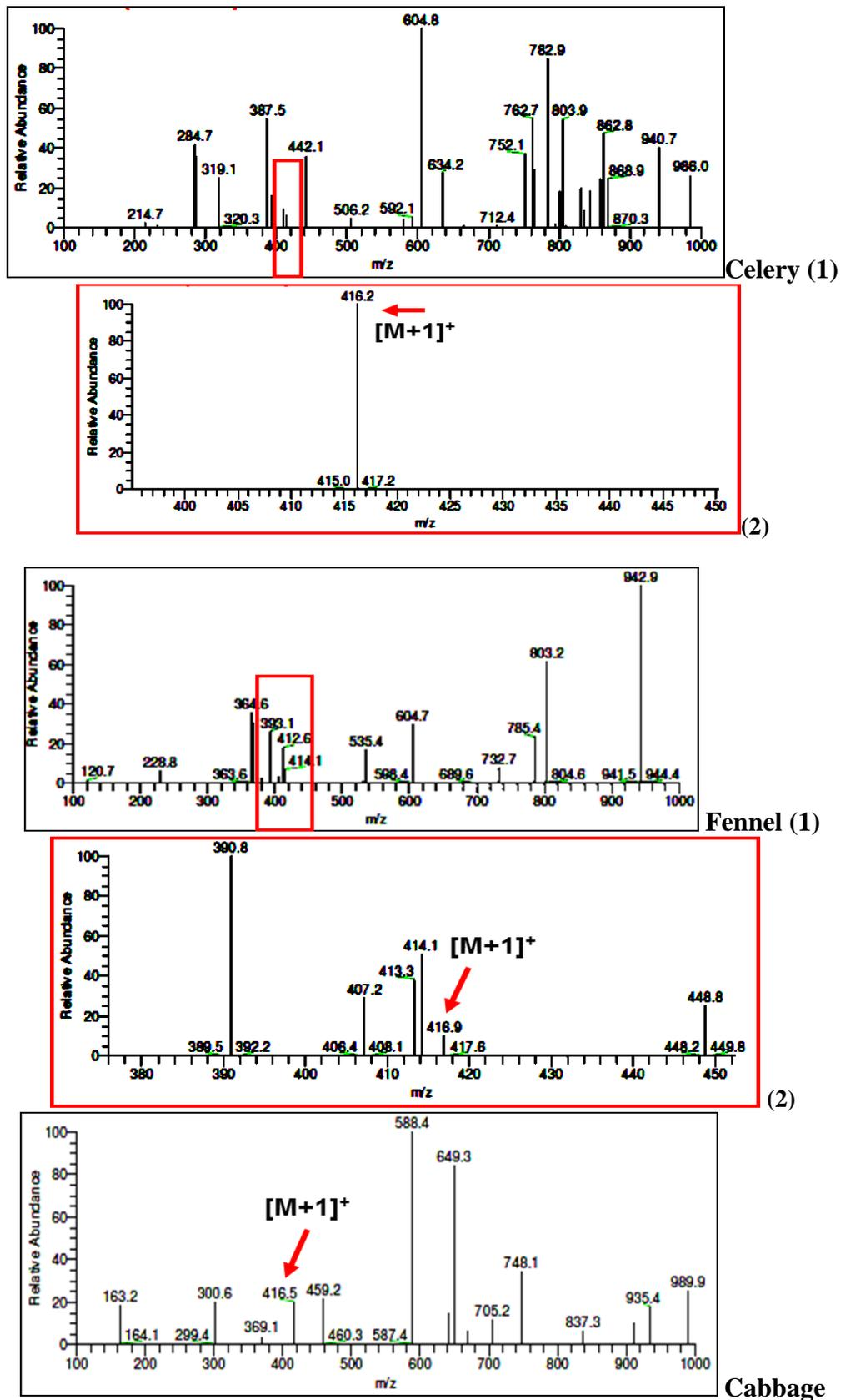
**Figure 5:** Detection of cypermethrin residues in vegetable samples treated with an illegal dose of the pesticide using LC-ESIMS analysis. 1: ESIMS of cypermethrin treated vegetable samples. 2: Expansion of MS region showing  $[M+1]^+$  of cypermethrin.
