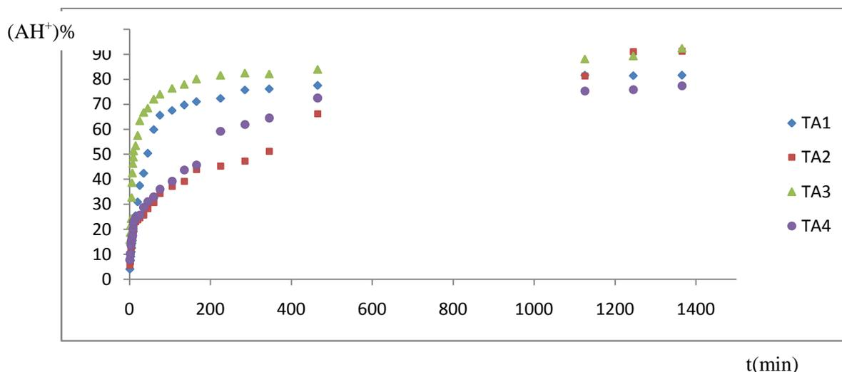
**Figure 7:** Release profiles of (AM) and (AMO) from microspheres (TA1, TA2, TA3 and TA4) in pH=1.2 at 37°C.
