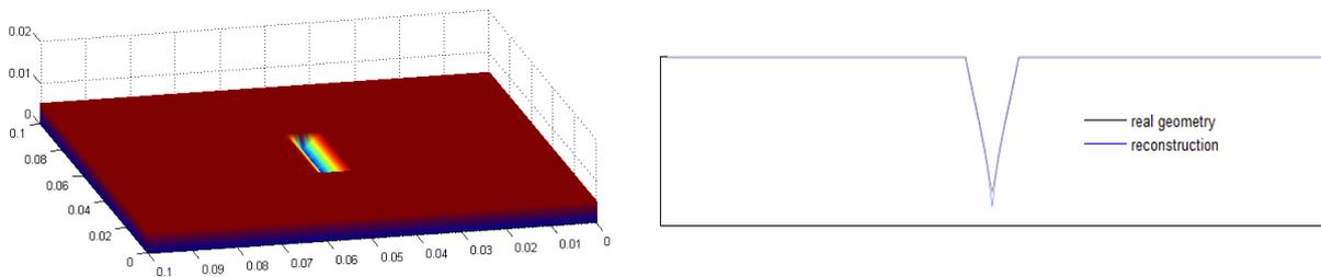
Fig. 6-a : 3D reconstruction of the triangular defect (left) and the corresponding section along the plane P1 (right).
