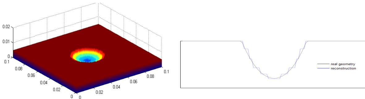
**Fig. 4-b :** 3D reconstruction of the elliptical defect (left) and the corresponding section along the plane P1 (right).
