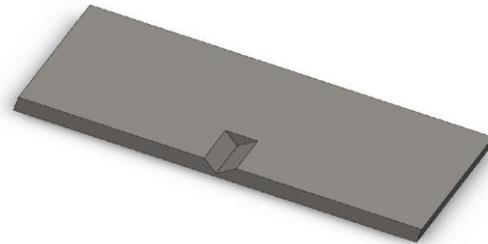
**Fig. 2-b:** Sample with triangular defect, Opening angle 90 °- Cutaway view
