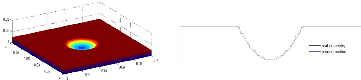
**Fig. 4-a :** 3D reconstruction of the elliptical defect (left) and the corresponding section along the plane P1 (right).
