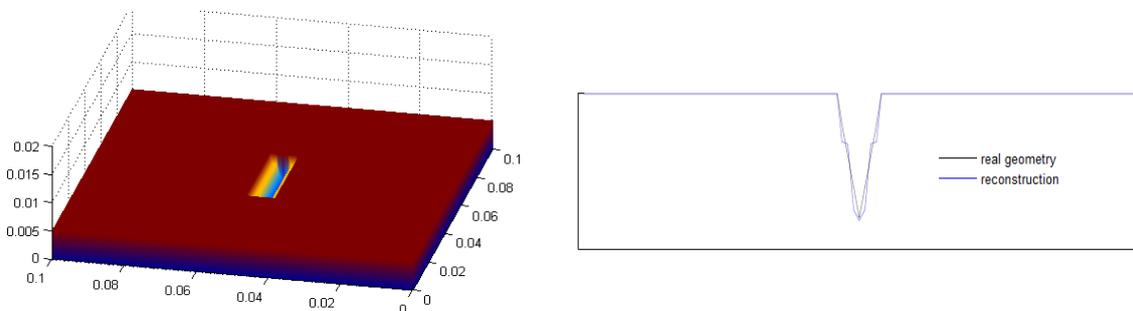
Fig. 6-b : 3D reconstruction of the triangular defect (left) and the corresponding section along the plane P1 (right).
