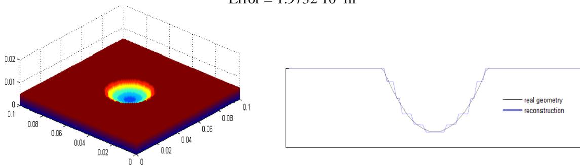
**Fig. 4-c :** 3D reconstruction of the elliptical defect (left) and the corresponding section along the plane P1 (right).
