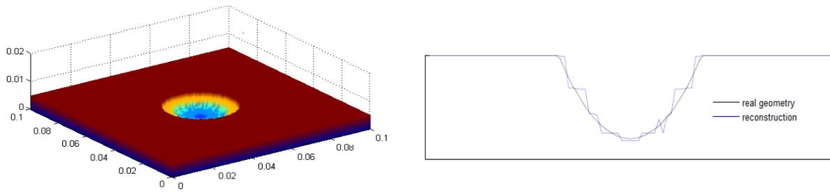
Fig. 5 : 3D reconstruction of the elliptical defect (left) and the corresponding section along the plane P1 (right).
