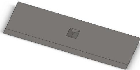
**Fig. 2-a:** Sample with triangular defect, Opening angle 90 °- Isometric view
