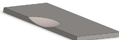
**Fig. 1-a** : Sample with an elliptical defect - Isometric view      **Fig. 1-b** : Sample with an elliptical defect - Cutaway view
