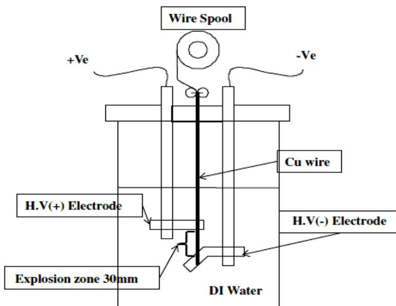
**Fig. 1:** Schematic pulsed wire explosion system used in is pulsed wire explosion technique [26].
