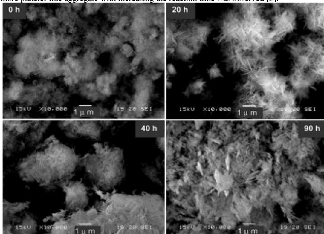
**Fig. 3.** SEM images of CuO nanostructures that changes from needle-like changes to fiber-like and then to a more platelet-like structure with changing the aging time of 0, 20, 40 and 90 h [5].
