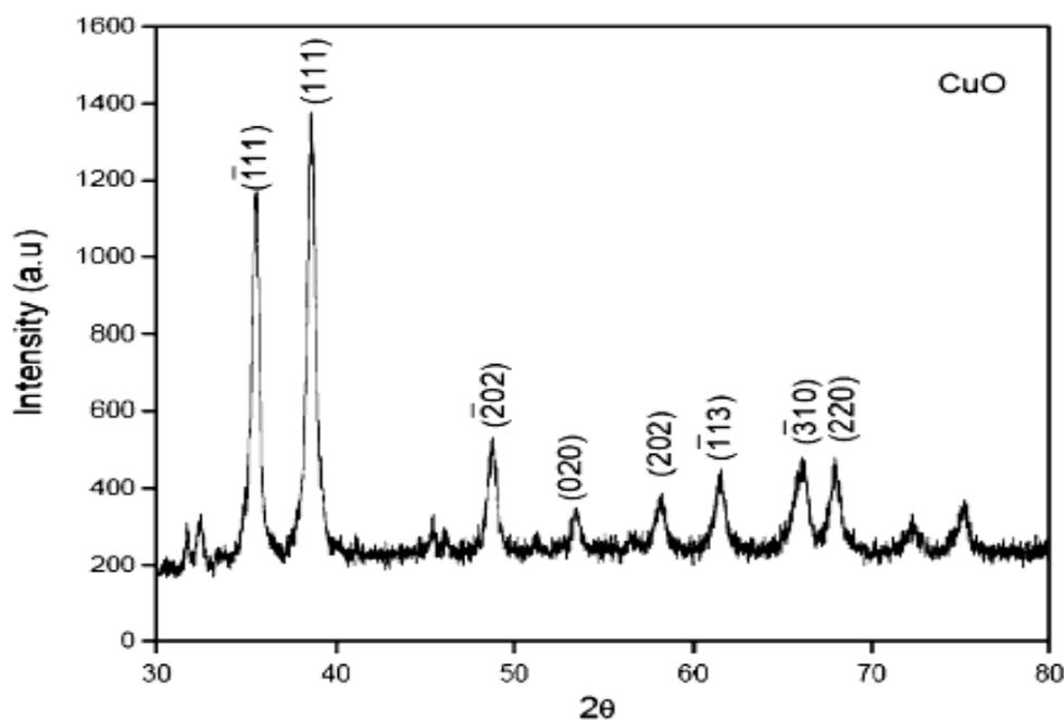
Fig. 4. XRD pattern of CuO nanoparticles.
