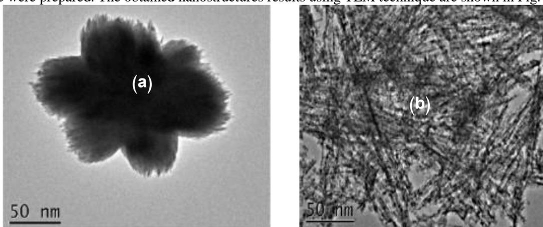
**Fig.2.** High resolution TEM images of different CuO nanostructures. (a) quasi-spherical microarchitectures and (b) long-straw like [1].
