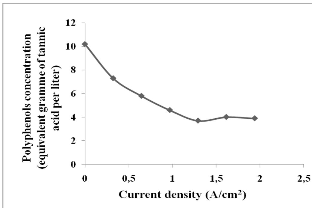
Fig.4: influence of current density on the elimination of the OMWW polyphenols by electrolysis on BDD electrode,  $t = 30\text{mn}$
