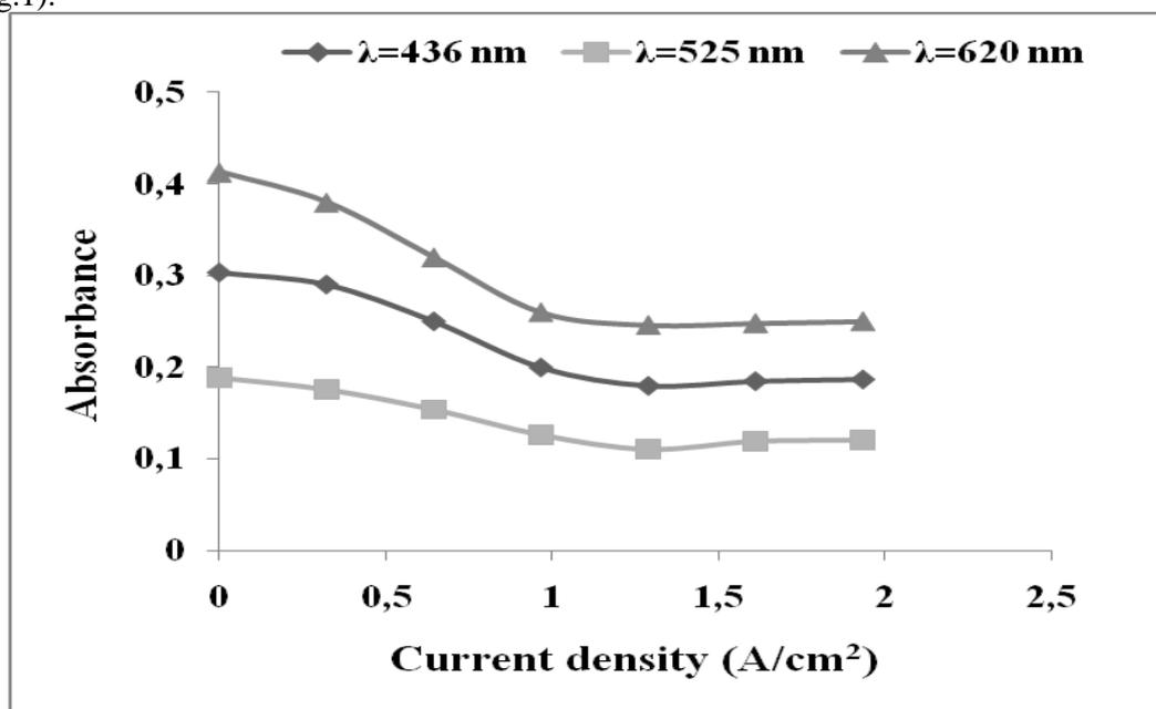
**Fig.1:** Coloration evolution during electrolysis on BDD electrode at different wavelengths, t = 30mn
