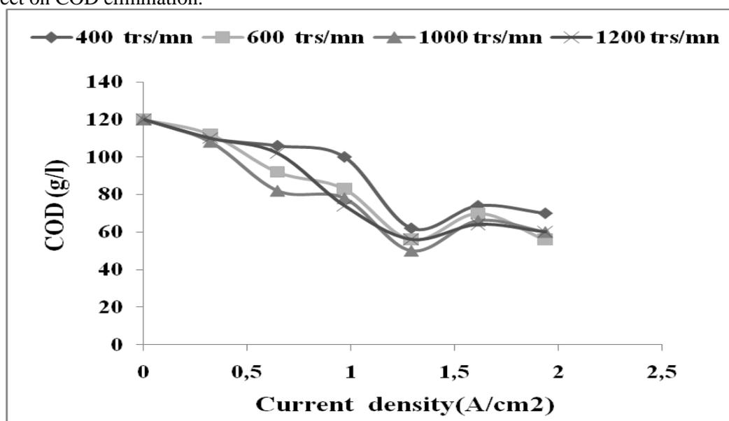
Fig.5 : Influence of electrode rotation speed on OMWW COD elimination by electrolysis on BDD electrode at different current density,  $t = 30\text{mn}$
