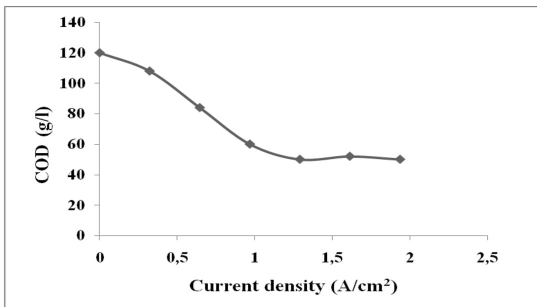
Fig.3: Influence of current density on the elimination of the OMWW COD by electrolysis on BDD electrode ;  $t = 30$ mn
