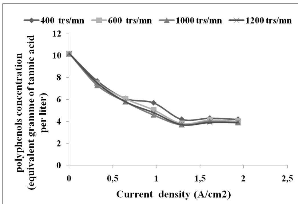
Fig. 6 : Influence of electrode rotation speed on OMWW polyphenols elimination by electrolysis on BDD electrode at different current density, t = 30mn
