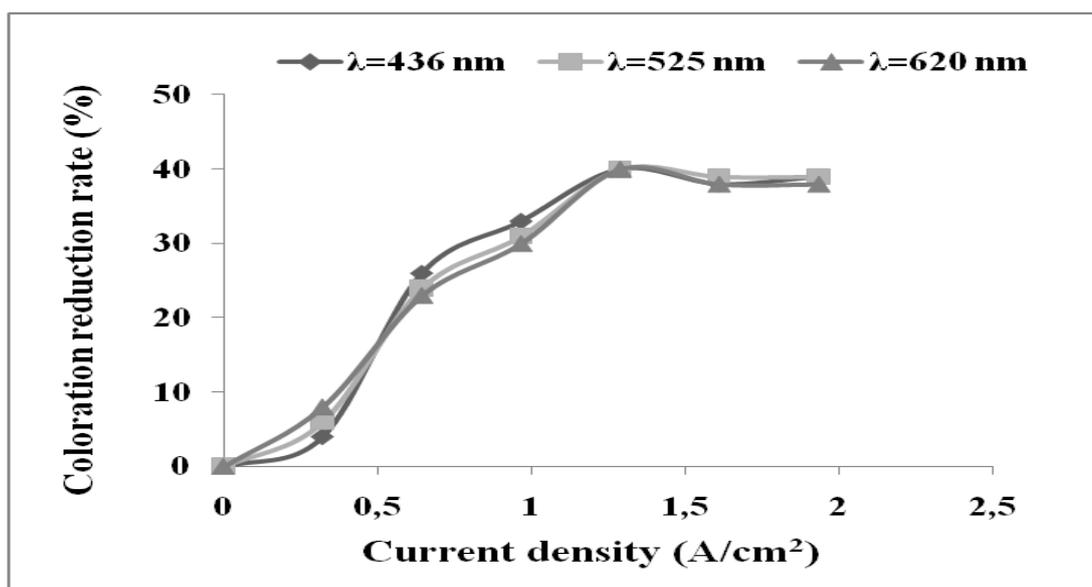
Fig. 2: Evolution of discoloration during electrolysis on BDD electrode at different wavelengths,  $t = 30$ mn
