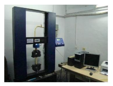
Fig. 3: Universal Testing Machine
