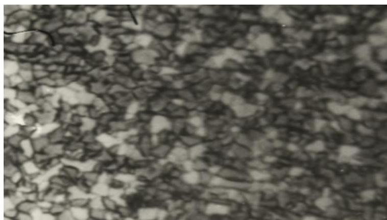
**Figure 13:** Optical Micrograph of Specimen SA-178A Coated with 1:3 (Vanadic Slag: MS) and fired at 950°C for 4h, using 500 times magnification.
