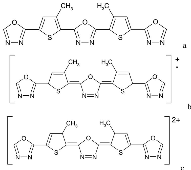
**Figure 5:** Simplified neutral (a), polaron (b) and bipolaronic (c) structures.
