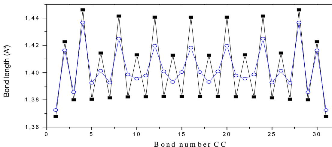
**Figure 4:** Optimized CC bond lengths of neutral compound OxTOxTOx(Me) (filled squares) and its diradical cation (open circles) calculated by the B3LYP/6-31G(d).
