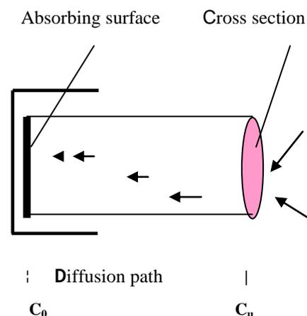
**Figure 2:** Principle of diffusion (samplers)
