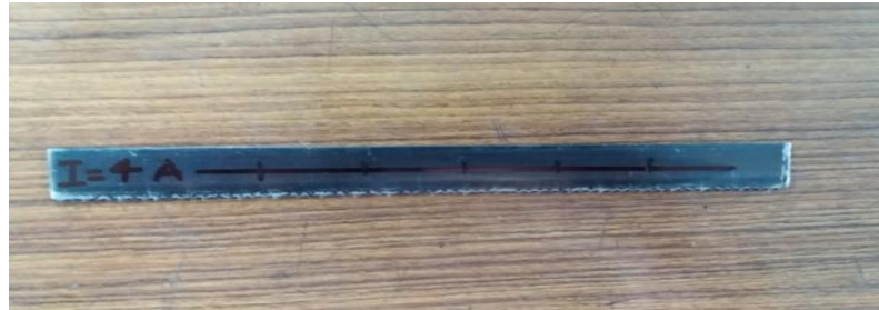
Figure 2. SK2MnCr4 carbon tool steel used for experiment
