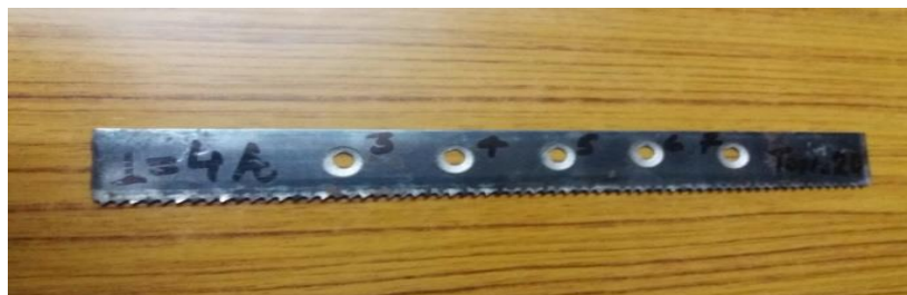
Figure 3. SK2MnCr4 carbon tool steel used for experiment for T_{on} (20 \mu s)
