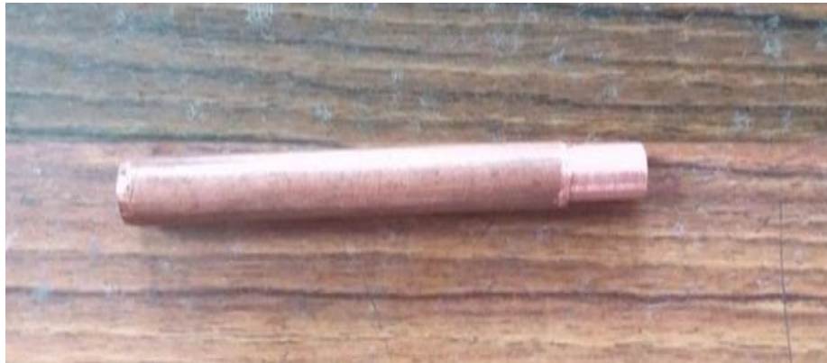
Figure 4. Copper electrode used for experiment
