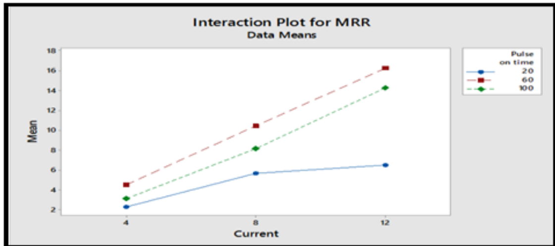
Figure 6: Interaction graph of MRR between current and pulse on time
