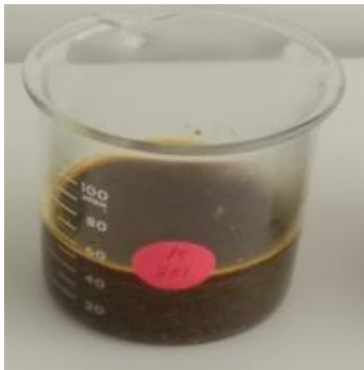
Figure 2. Nano-silica gel based on river sand
