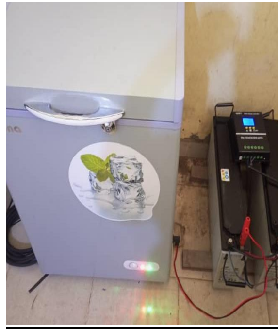
Figure 4: Temporal Set-up of Solar panel and DC FREEZER with batteries and charge controller
