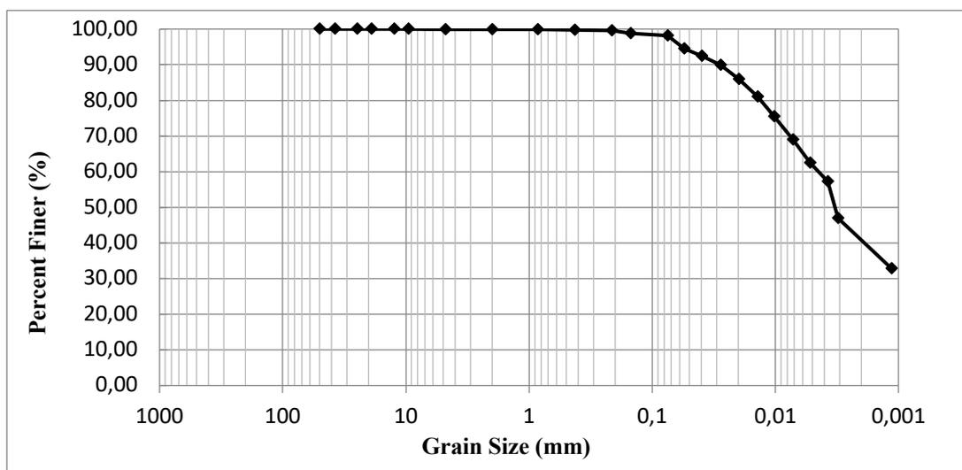
**Figure 1:** Grain size distribution of clay soil sample
