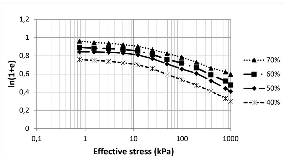
Figure 5: The effective stress vs  $\ln(1+e)$
