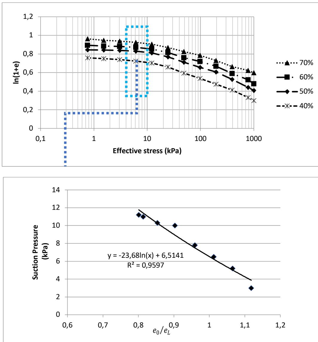
**Figure 9:** suction pressure vs  $e_0/e_L$
