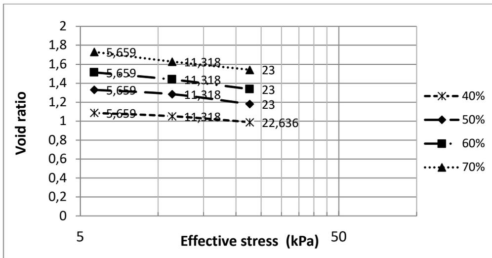
Figure 3: effective stress vs void ratio (preloading stage)
