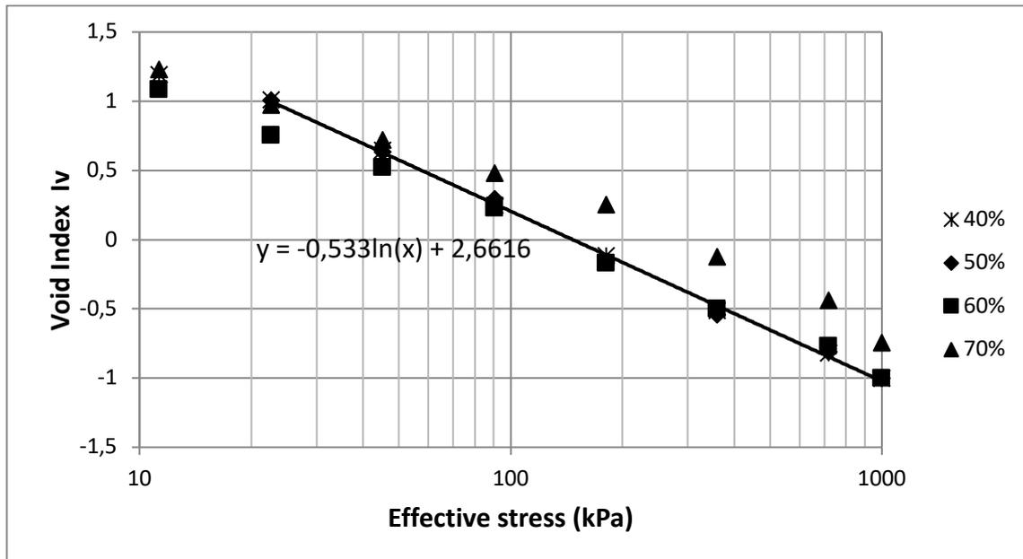
**Figure12:** effective stress vs void index  $I_v$
