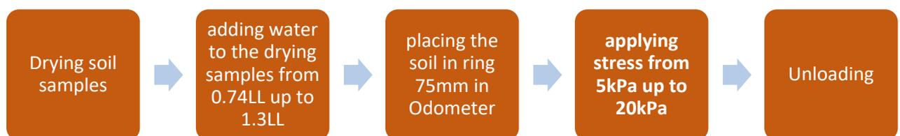
**Figure 2:** scheme of reconstituting steps of clay sample
