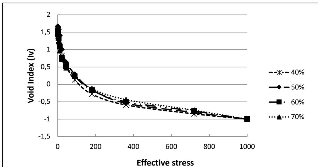
**Figure 11:** effective stress vs void index  $I_v$  ( $\sigma' > \sigma'_s$  kPa)
