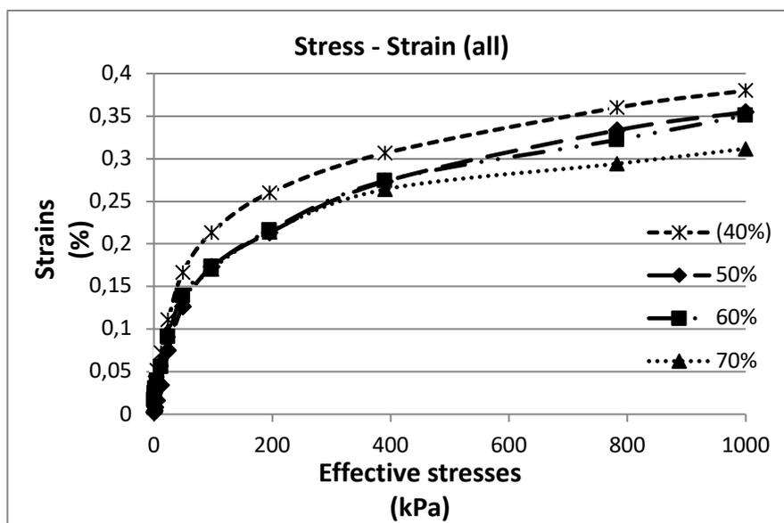
**Figure 6:** Stress vs strain after consolidation
