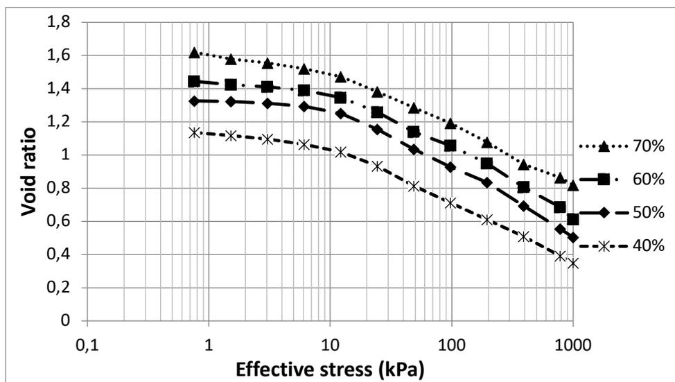
Figure 4: The effective stress ( $\log \sigma'_v$ ) vs void ratio after Oedometer test for reconstituting samples
